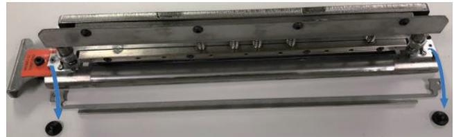
3. Turn the die onto its side and unscrew the 3 knurled screws from the underside of the die.
