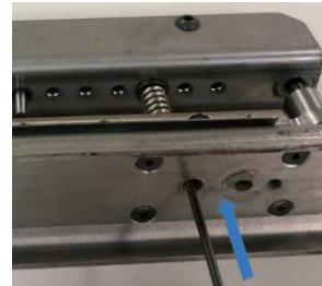
5. Slide the new backing plate into the throat of the die and let it fall into the backing plate opening.
