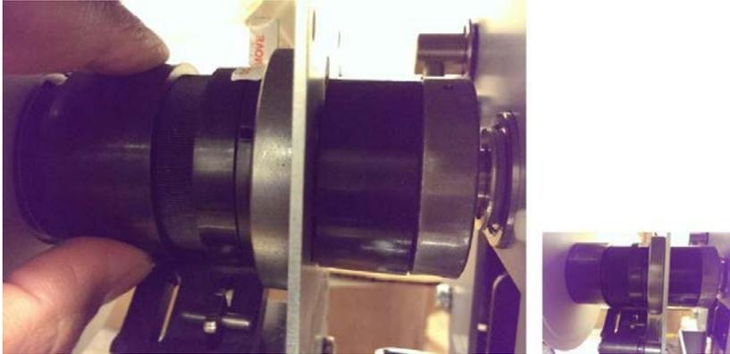
If the Punch Cam needs to stop earlier, rotate the Stop Collar Clockwise (when viewed from the rear of the machine).
