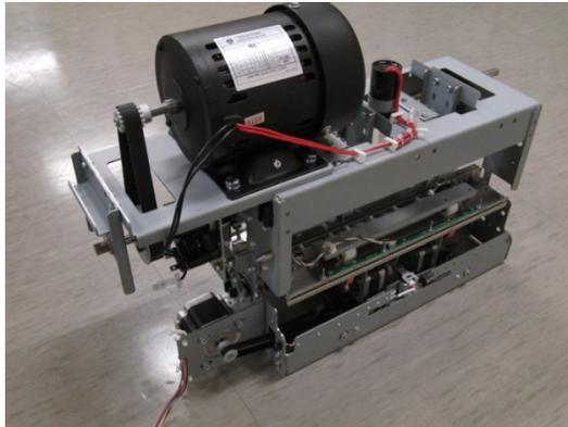
4. Remove the E-Ring from the Steering Drive Roller shaft from the side that needs to be replaced and the two e-rings in side the bracket.
