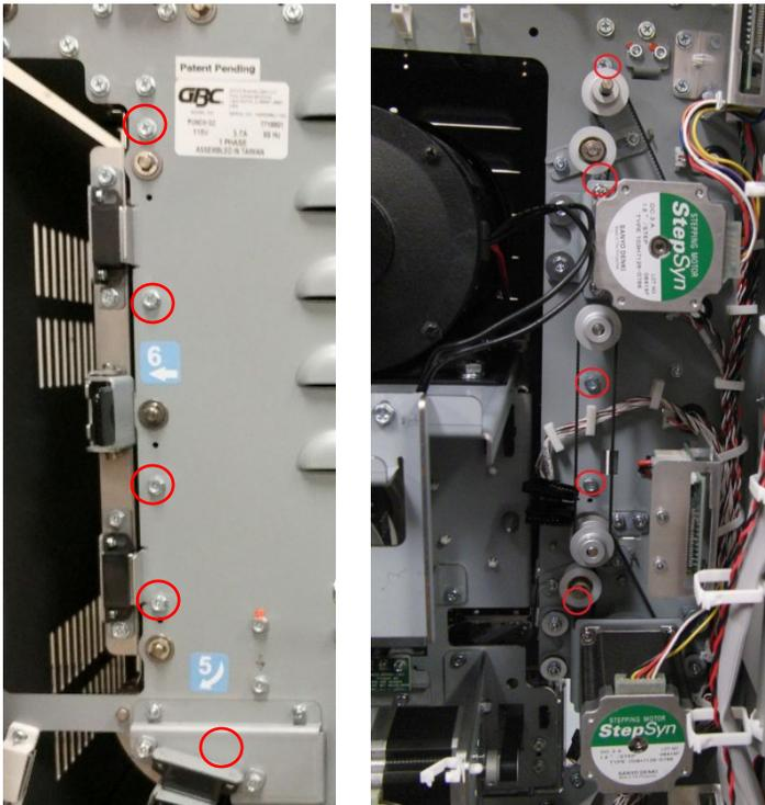
2. Using the Reference holes in the front/rear frame (4 holes in the front frame and 4 holes in the rear frame) and the sheet metal panel, position the drive panel to ensure the drive rollers protrude  $1.5 \pm 0.5 \text{ mm}$  through the drive panel.
