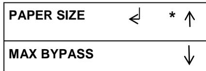
2. Press the down arrow button to move the return symbol next to MAX BYPASS. Press OK to enter the Max Bypass setting
