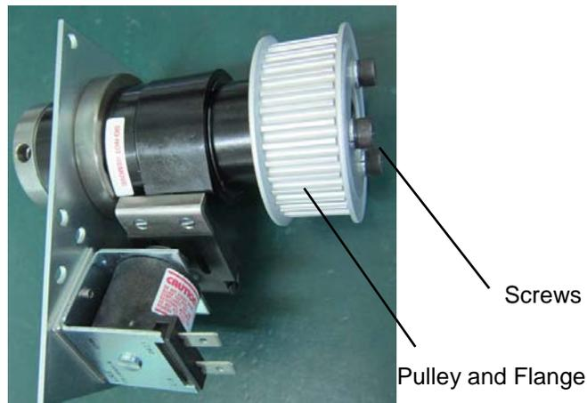
6. Remove the Lock Nut and the long M6 Screw.
