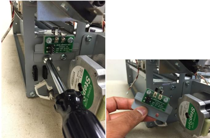
5. Place the Dieset Recognition Reader Board in position and tighten the Screws (2).
