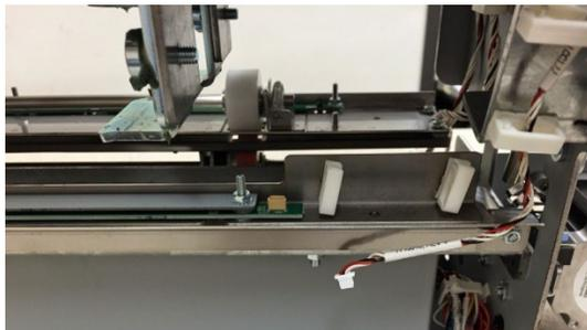
7. Transfer the Backgage Sensor and all fasteners to the new part.
