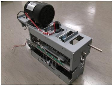
6. Remove the Shoulder Screw from the hole in the Shaft at the rear of the Punch Module.
