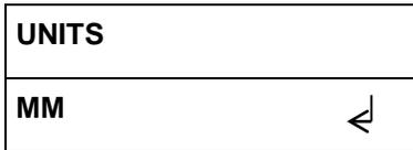
5. Press either the up arrow button or the down arrow button to change units from mm to inch or vice versa.
