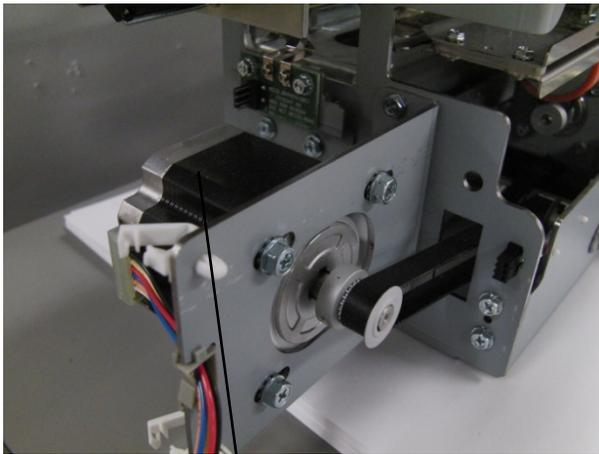
Punch Alignment Stepper Motor (M5)
