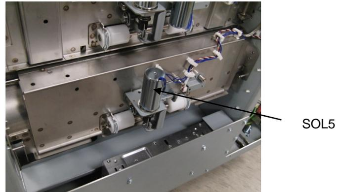
5. Open the Cable Clamps and remove the Cable.
