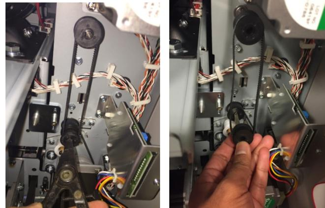
4. Place the Belt in position between the Pulleys and slide the Pulleys on to the Shafts.
