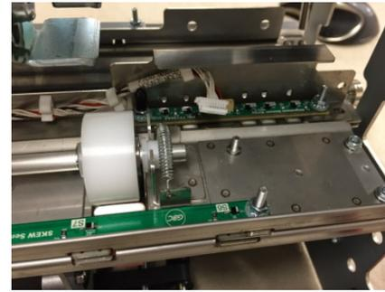
7. Remove M3 Nuts (2) that hold the Brackets.
