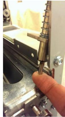
6. Inspect (4) plastic bushings in the Die lock brackets. (2) in the front and (2) in the back.
