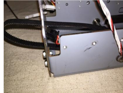
10. Remove the Phillips Screws (8)- (4) from front side and (4) from rear side
