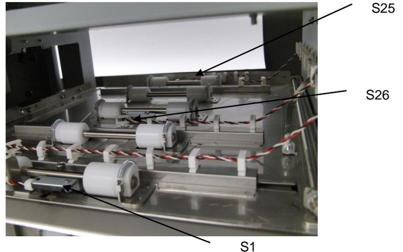
3. Disconnect the Sensor Connector at the Sensor.
