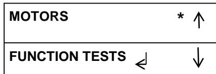
3. Press the ENTER button when the return symbol is next to the words FUNCTION TESTS to display the display the FUNCTION TESTS screen.
