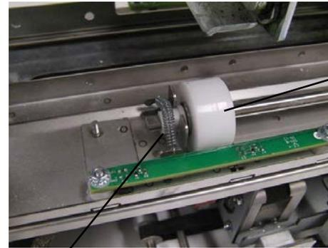
3. The roller surfaces should be free of debris, toner deposits, wear, unevenness, and dents.
