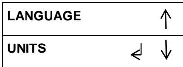
4. Press the ENTER button when the return symbol is next to the word UNITS to display the UNITS screen.
