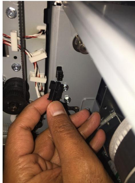
16. Disconnect the Connector for Punch Motor M10.
