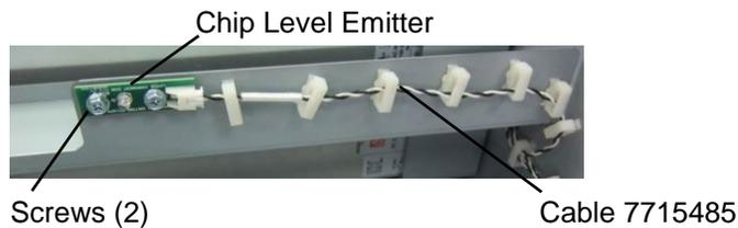
6. Remove the Screws (2) and the old Chip Level Emitter.
