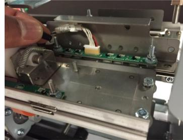
8. Disconnect the Alignment sensor board connector.
