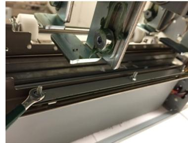
6. Place the new Backage Sensor Board in position.
