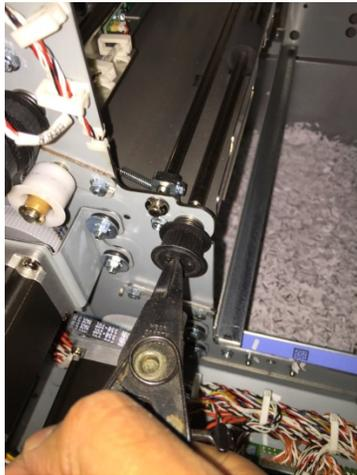
6. Remove the Belt from the Motor Pulley
