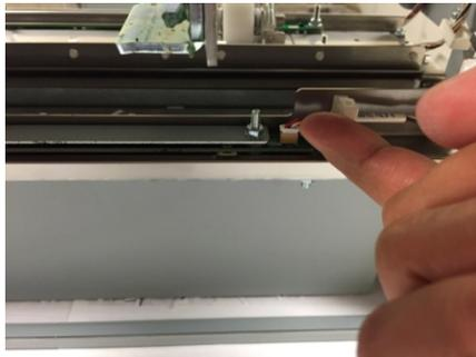
5. Remove the Nuts (3), Washers (3), and the Backage Sensor Board.
