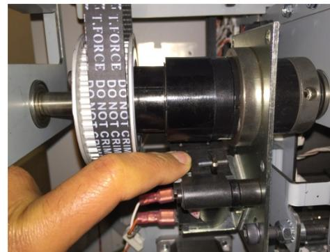
8. Remove the Clutch from the Shaft.
