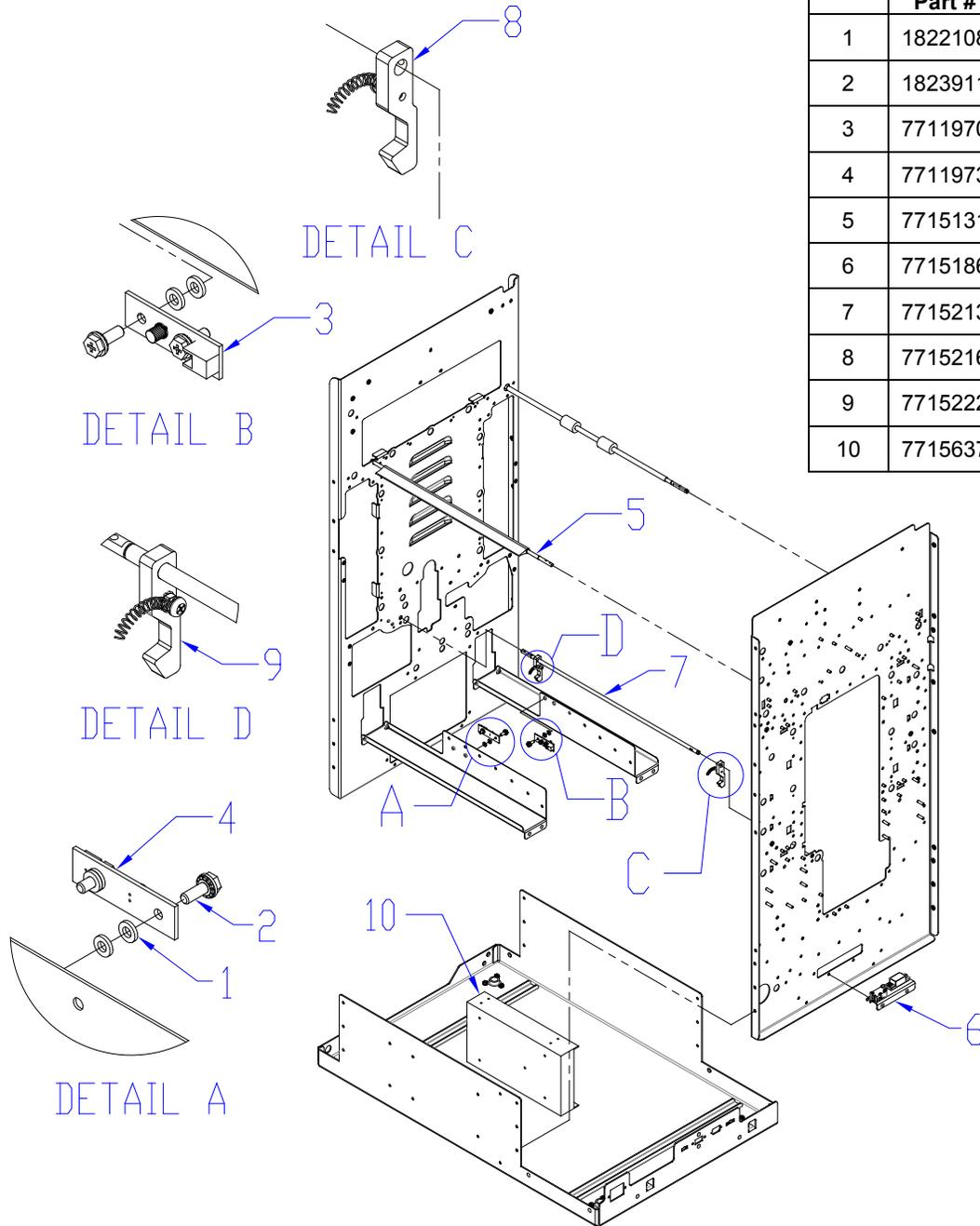
**PL 2.6. Frame Assembly- Motors and Motor Drivers**
