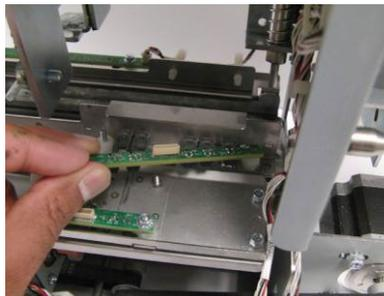
12. Place the new Alignment Sensor Board in position.
