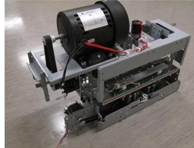
4. Do GP 6.3 *Undock the Punch* to separate the Punch from the upstream and downstream devices.
