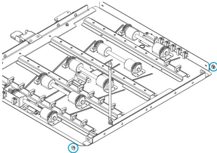
3. Remove the Snap-in Bearing.
