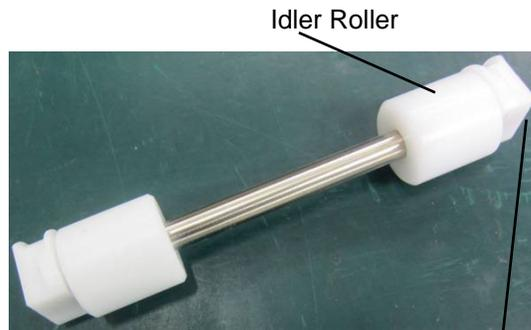
2. Remove the old Bearing Housings (2) from the ends of the Shaft.
