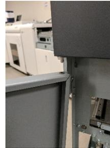
2. Insert the bottom door pin into the Front Door Bottom Hinge Bracket
