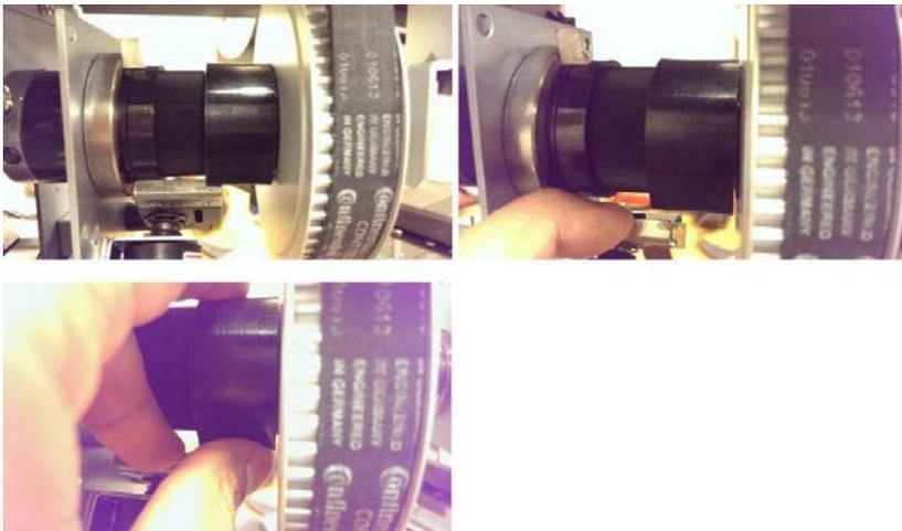
11. Slide the Stop collar back to its position and release the pawl.
