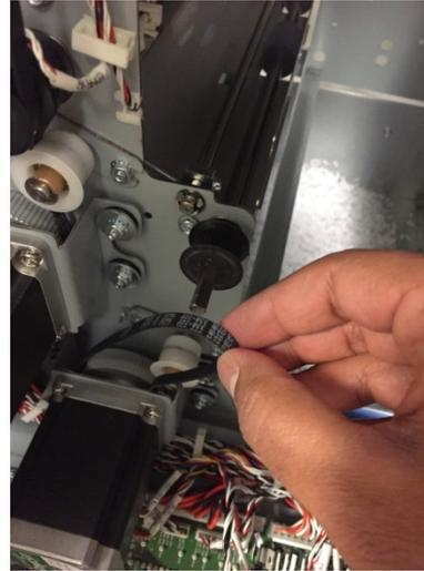
7. Slide the Pulley off the Roller Shaft.
