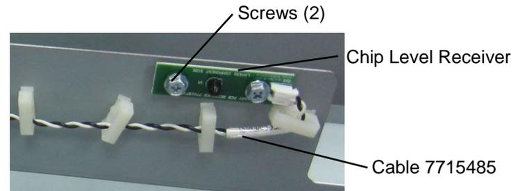
6. Remove the Screws (2) and the old Chip Level Receiver.
