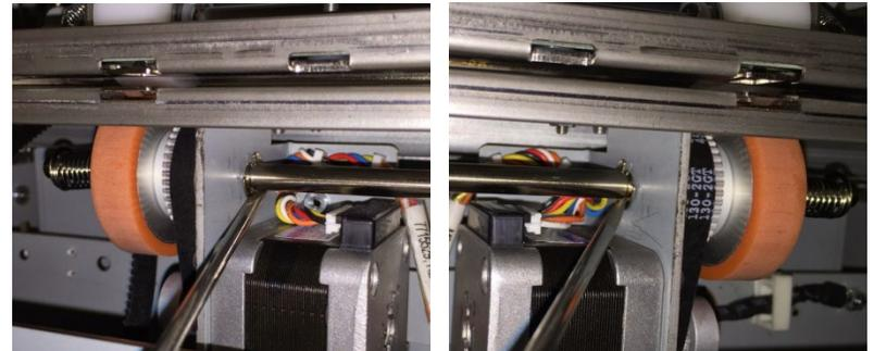
5. Slide the Shaft in the opposite direction so that the Steering Drive Roller Spring, (2) plastic washers and Steering Drive Roller can be removed (from the side that needs the part replaced).
