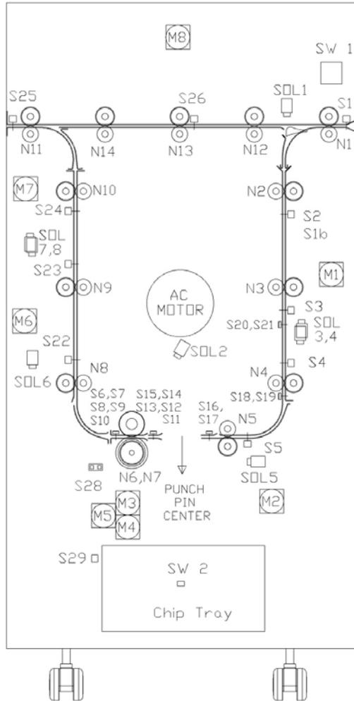
If the Punch is enabled, the transport and punch motors are started, and the Divert Solenoid SOL 1 is activated to direct the sheets into the punch path.
