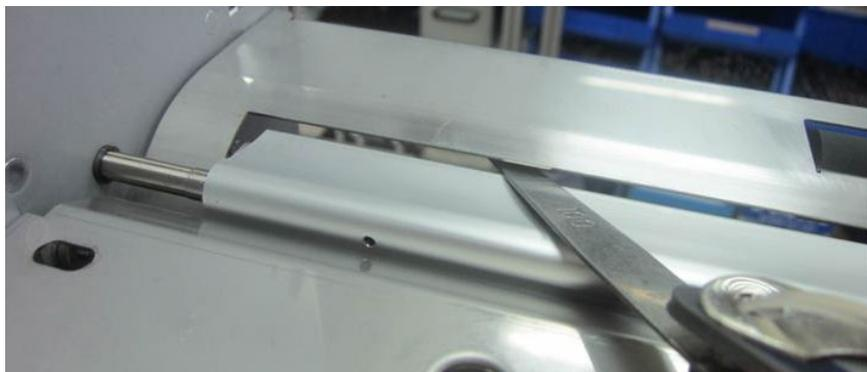
The clearance should be minimum 1.0 mm.
