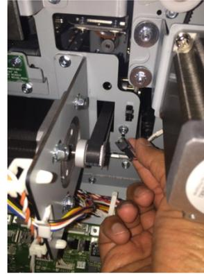
11. Disconnect the Connector for Solenoid SOL2.
