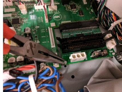
5. Disconnect the Connectors (29) from Main and Comm boards.
