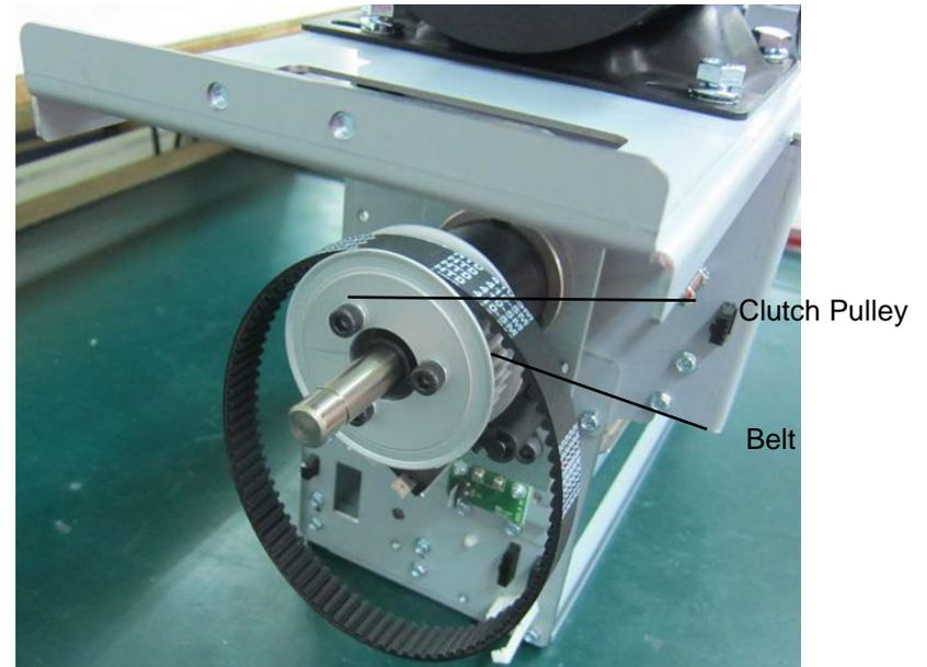
9. Place the new Belt around the Timing Pulley on the Punch Motor and the Clutch pulley.
