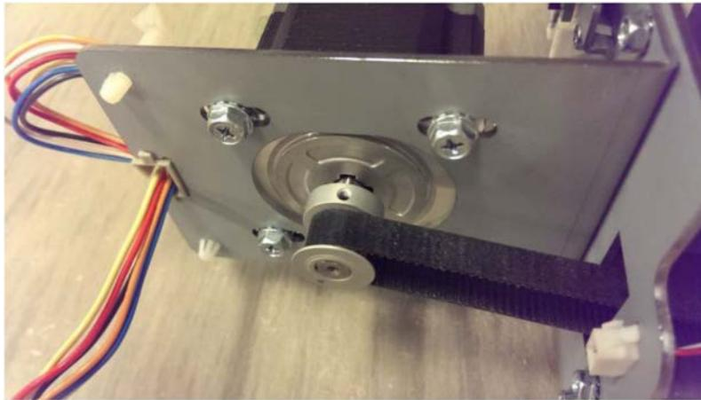
**The set screws are secured tightly.**
