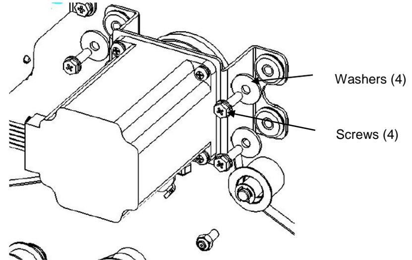
7. Place the Stepper and Mount Assembly in position and tighten the Screws (4).
