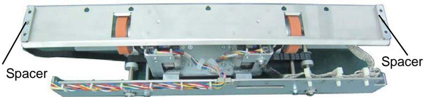
5. Remove the Nuts (4) holding the Steering Drive Panel Weldment.
