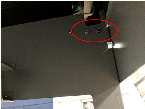
5. Place the new Front Door Top Hinge Bracket in position and tighten the Screws (2).
