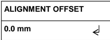
5. Press the up arrow button or the down arrow button to change the offset by  $\pm 0.1$  mm.
