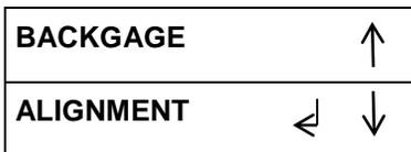
4. Press the ENTER button when the return symbol is next to the word Alignment to display the ALIGNMENT OFFSET screen.
