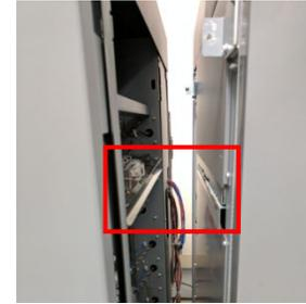
To adjust the casters, loosen the top nut on the caster, and rotate the wheel by hand. Clockwise to lower, counterclockwise to raise. Once the desired height is achieved, tighten the top nut to secure the caster.
