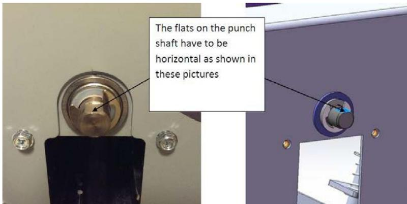
2. If the flats are not horizontal ( $\pm 5^\circ$  from horizontal is acceptable), do the following procedure to set the shaft indexed position.
