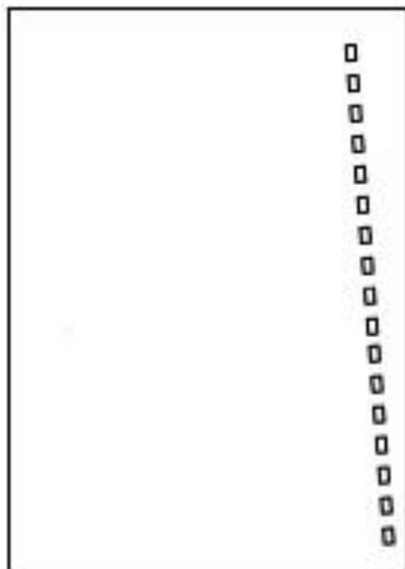
Top most hole is at correct Backgafe depth, but the bottom hole is too far from the edge of the paper.
