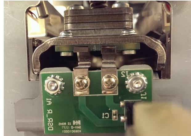
If Spring Clips are broken, Replace Dieset Recognition Reader Board. If the springs clips do not contact the Dieset Recognition Board, do ADJ 1.6 Dieset Recognition Board Adjustment.
