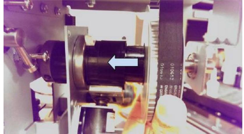
12. Manually rotate the pulley in the counter-clockwise direction by holding the pulley (viewed from rear side) to complete a punch cycle.
