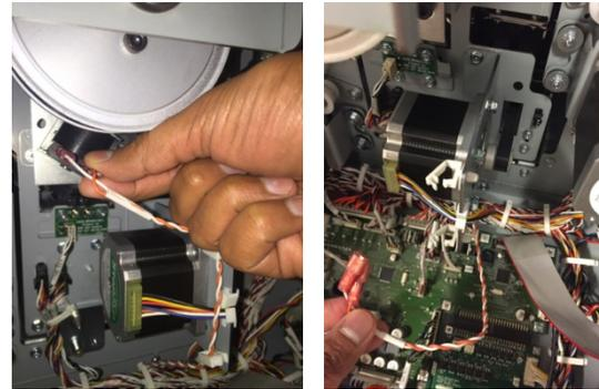
12. Disconnect the Connector for the M5 Motor Driver.
