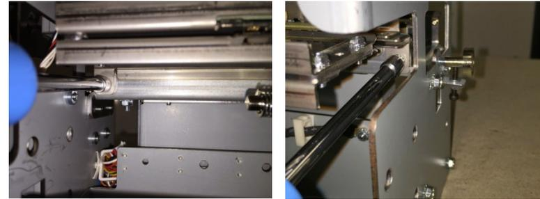
8. Remove both upper and lower brackets as shown, do not pull on the Align sensor wires.
