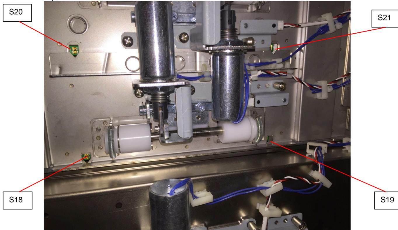
Sensors S18 and S19 are on Mid Punch Large Backgage Sensor Board.
