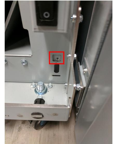
Once the brackets are aligned with the holes in the PUNCH G2, push the punch back so that it engages the alignment pins. Install item 10 in the lower right front bracket and secure the upper bracket using a M4 screw.
