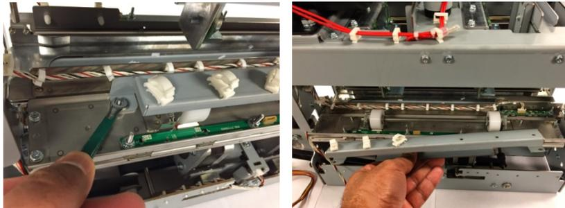
7. Remove the sleeve from the threaded stud.
