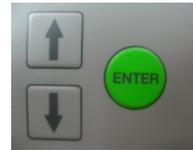
Then while still holding down the Up Arrow button and the Down Arrow button, press the Enter button.
