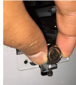
5. Tighten the Nut and Lock Screw.
