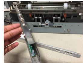
10. To replace the upper bracket, remove the cable clamps, cable, Alignment sensors, washers, nuts from the old bracket and transfer them to the new bracket.
