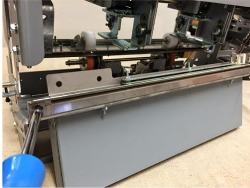
10. Remove Nuts (3) and the Chip Chute.
