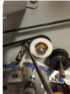
6. Slide the Diverter Assembly to the back side and remove the part.
