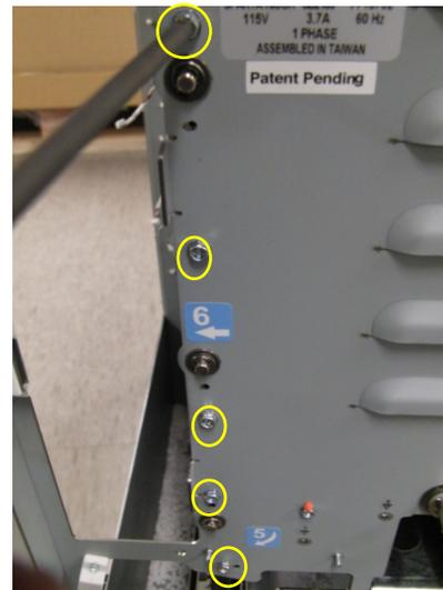
10. Remove (5) screws from the rear frame that mount the Exit drive panel.
