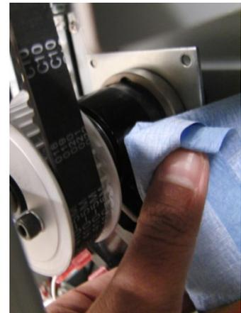
7. Inspect the collar stop and the metal insert pawl for any wear.
