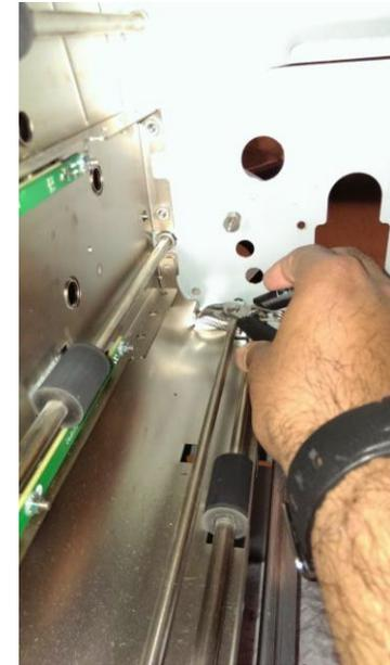
5. Remove the M3 screws (2) from the Accel Idler Panel Front and Rear Latches.
