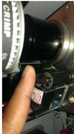
8. Check the tightness of (2) cone point set screws in the clutch.
