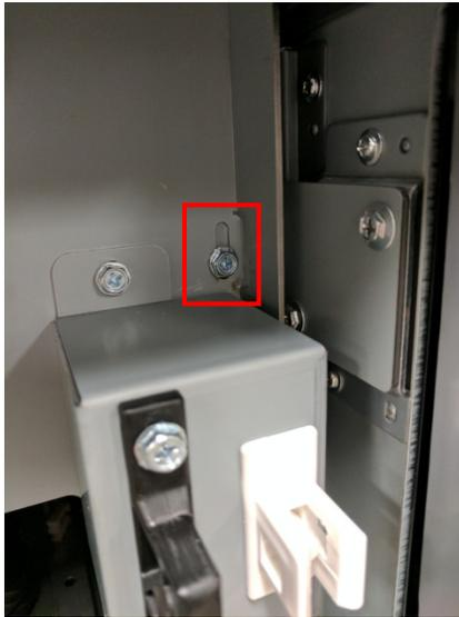
Remove the two M4 screws from each spacer. The spacers are held to the PUNCH G2 with adhesive and should remain in place. Use these screws to secure the brackets provided with the downstream device. See the Konica Minolta Installation manual for more details.
