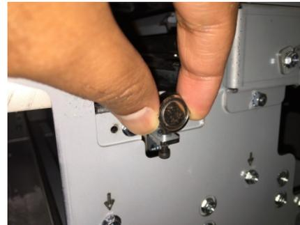
4. Place the new Die Set Magnet on the Shaft and rotate it clockwise.
