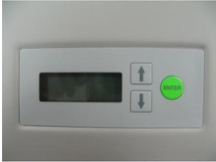
The buttons on the User Interface allow you to change the backgauge, alignment, language, and the units.
