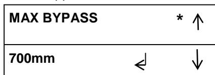
4. 1260mm is the Max Bypass setting. To reduce the Max Bypass setting, press the down arrow to the desired setting, and then press OK.
