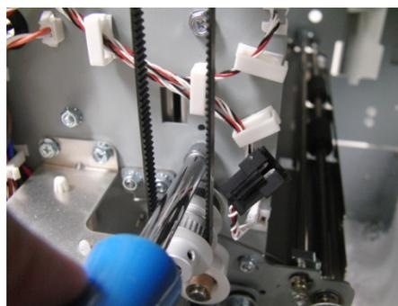
12. Remove the Screws (5) that hold the Entrance Drive Panel to the Rear Frame.
