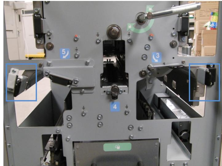
6. Remove the M4 X 10 Phillips Head Screw and the Die Lock Handle.
