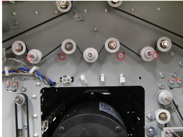
2. Using the Reference holes in the front/rear frame (4 holes in the front frame and 4 holes in the rear frame) and the sheet metal panel, position the drive panel to ensure the drive rollers protrude  $1.5 \pm 0.5$ mm through the drive panel.
