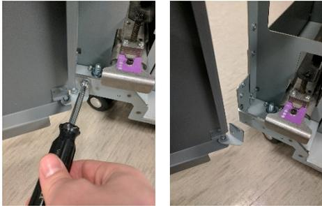
4. Lower the Door down off the pin on the Front Door Top Hinge Bracket.
