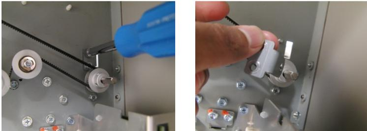
10. Remove the Upper Bypass Assembly.
