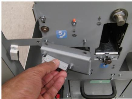
7. Do ARP 2.27 to remove Motor M7 by removing (4) screws.
