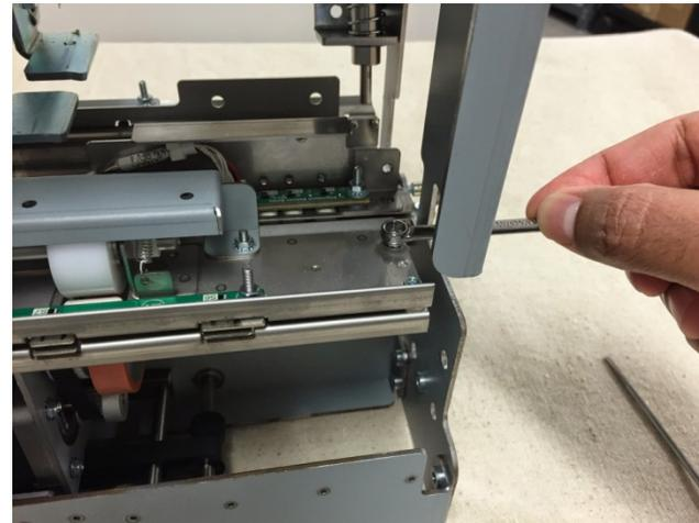
6. Remove the Steering Idler Panel Sub Assembly.
