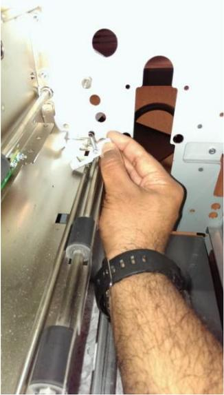
11. Remove Accel Panel Rear and Front Latch assemblies to remove the Accel Idler Latch shaft.
