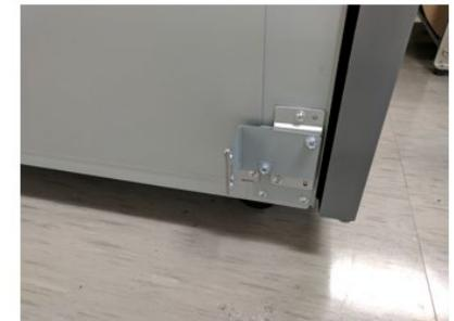
5. Remove the Docking Brackets from the upstream device.
