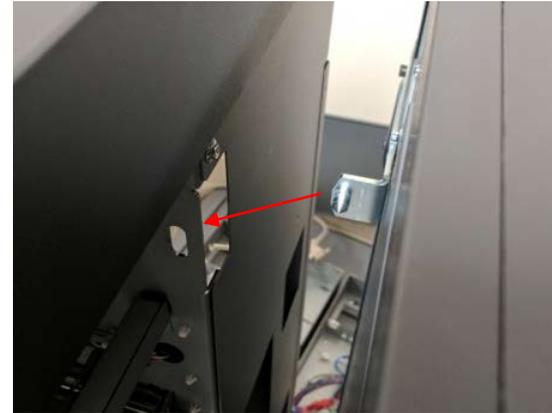
2. Slide in the upstream and downstream docking mechanisms and install the locking screws.
