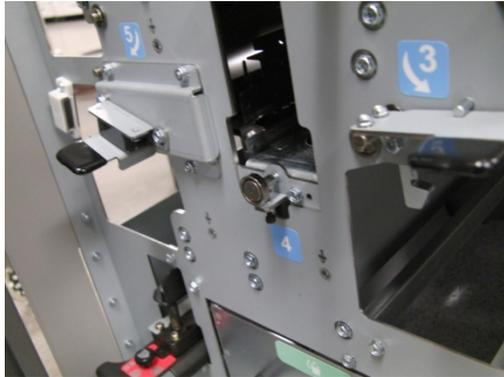
3. Loosen the Nut and Lock Screw.
