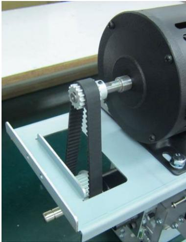
10. Place the Bearing Bracket in position and tighten the Screws (2).
