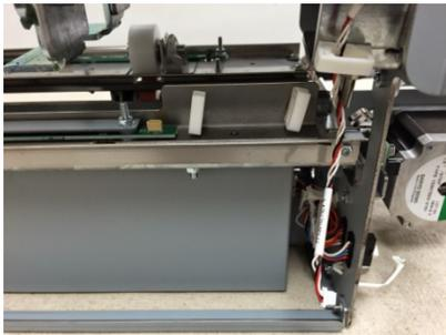
6. Remove the Screws (2) that hold the Diesel Recognition Bracket.
