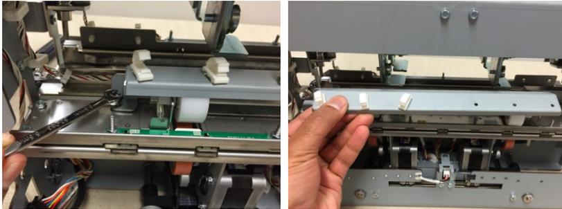
6. Unplug the Alignment Sensor Connector
