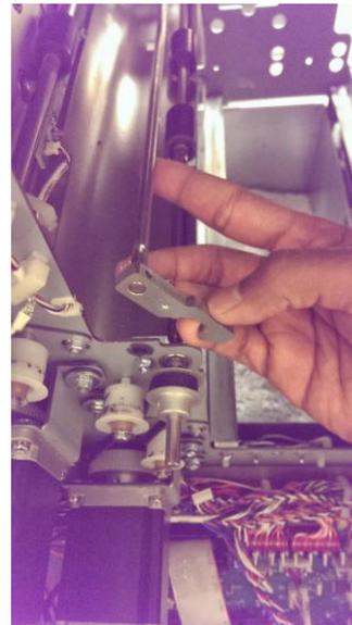
10. For the Accel Idler Panel Front Latch Assembly, slide the shaft towards the rear side to remove.
