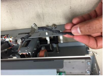
8. Remove the Steering Carriage Ground Strap.
