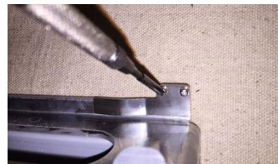
Remove the backage sensor upper and lower brackets.
