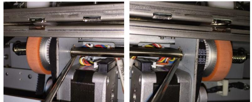
6. Remove the Shaft from the Drive Panel Steering Sub Assembly.
