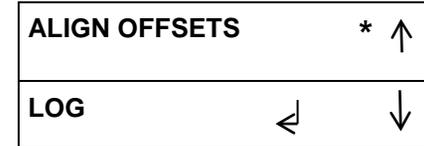
5. Pressing OK when the return symbol is next to LOG will open the LOG file capture option.
