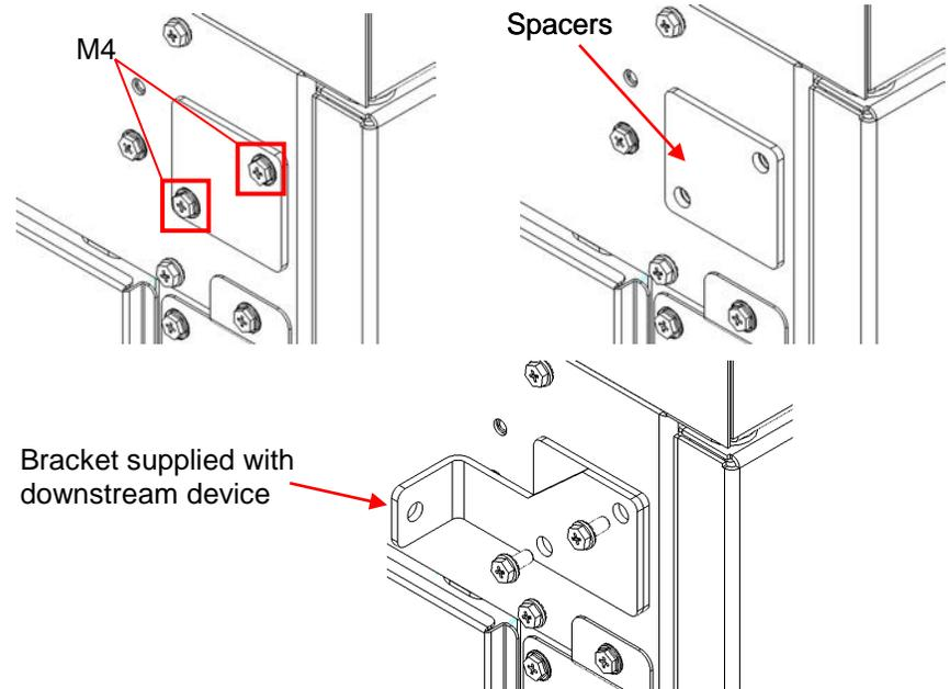
The PUNCH G2 comes with four spacers installed for the mounting of the downstream brackets.
