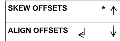
3. Press the ENTER button when the return symbol is next to the words ALIGN OFFSETS to display the ALIGN OFFSETS screen.
