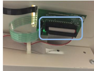
**Cable 7715523 is connected at the LCD Panel.**
