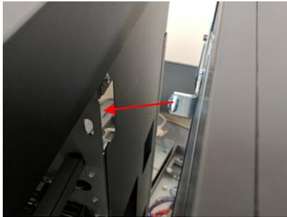
The upstream docking brackets should align with holes in the PUNCH G2
