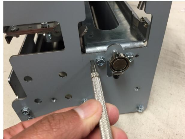
7. Tighten the Screws (2) that hold the Dieset Recognition Bracket.
