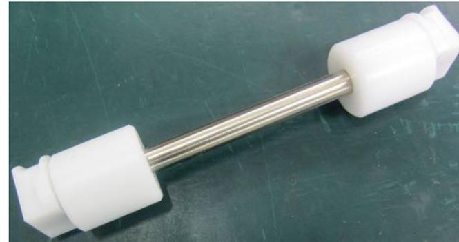
5. Remove the Bearing Housing (2) at each end of the Idler Roller Shaft.
