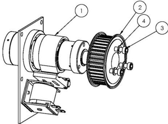
11. Place the Punch Shaft Bearing Bracket in position and tighten the Screws (2).
