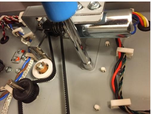
7. Remove the Diverter Solenoid Sub-assembly.
