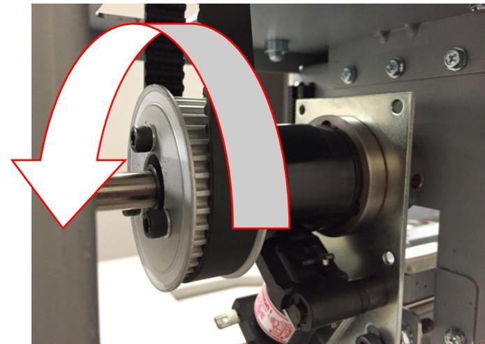
13. Repeat Steps 10 to 13 until the Punch shaft flats are horizontal. It is important to turn the punch shaft with a wrench until it hits a hard stop in the counter-clockwise direction (viewed from rear side). Important note: Turning the shaft with hand will not provide enough torque and the setting will be incorrect. Therefore use a wrench to turn the shaft.
