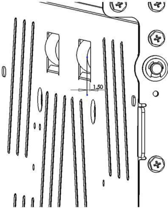
1. To adjust the position of the drive panel loosen (5) screws from the Front frame and (5) screws from the rear frame.
