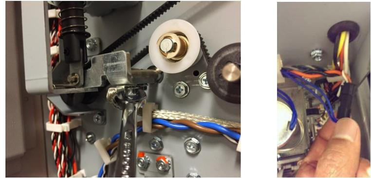
5. Disconnect the inline Connector for the Diverter Solenoid sub-assembly.
