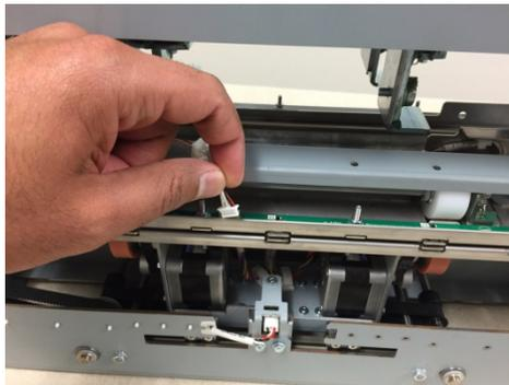
5. Release the Cable Clamp and move the Cable out of the way.
