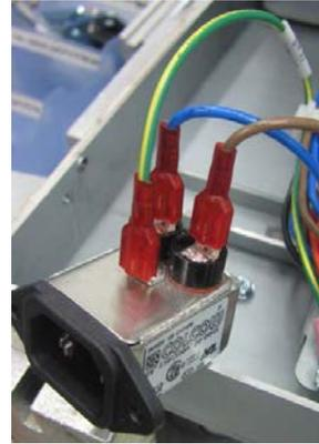
5. Remove the Wires (3) and the AC Filter.
