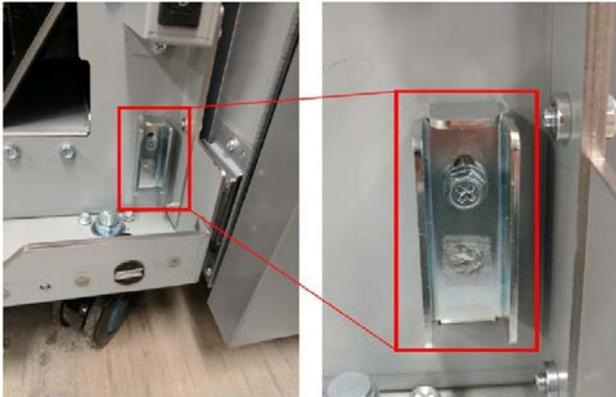
4. Pull on the punch forward to disengage the locking pins.
