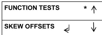
3. Press the ENTER button when the return symbol is next to the words SKEW OFFSETS to display the SKEW OFFSETS screen.
