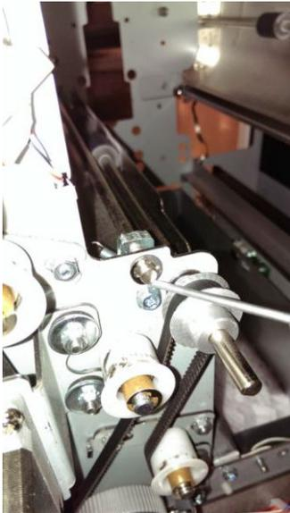
7. Do ARP 2.20 to remove the Accel Idler Latch Handle.
