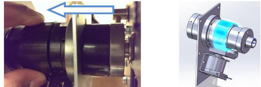
For some 230v machines, moving the stop collar towards the pulley may not expose the teeth completely. In such instances, remove the pulley off the clutch (3 sets of socket head screws and washers), see ARP 3.7 Clutch Pulley replacement.
