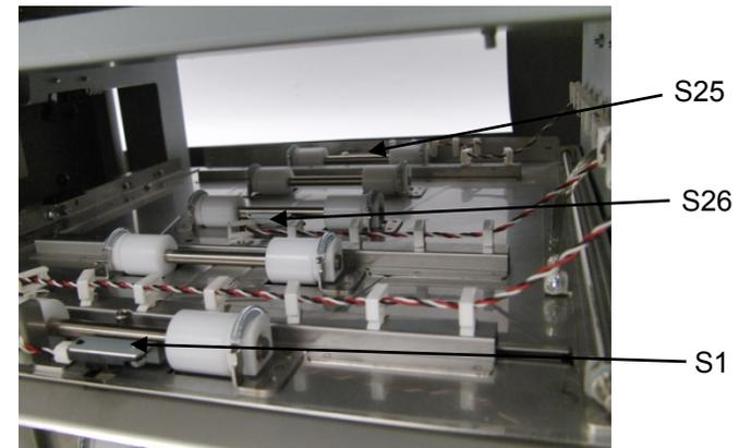
**PL 3.6. Paper Path- Disengaging Roller Solenoid**
