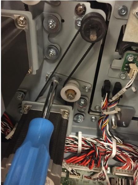
4. Place the new Belt in position around the Pulleys.
