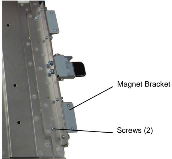
5. Place the Magnet Bracket in position and insert the Screws.
