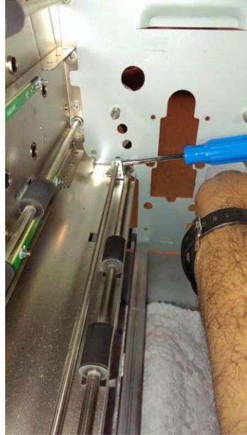
6. Remove the E-clip from the Accel Idler Shaft on the rear side.
