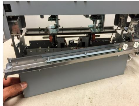
9. Die rail springs can be replaced at this point by unscrewing M2 screws (4) and M2 lockwashers (4). If you are replacing only the springs, go to Installation procedure.
