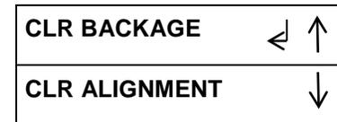
This displays the CLR BACKGAGE screen. Enter the desired value, the Offsets are in +/-0.2mm increments
