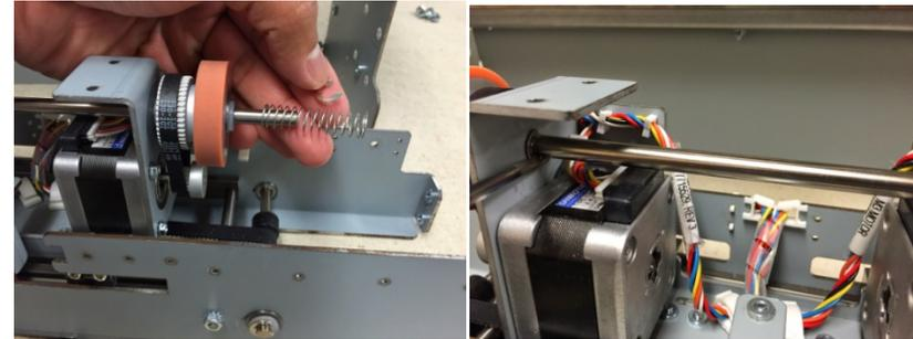
7. Remove the drive roller shaft and all the components on the drive shaft. (4 plastic washers; 2 springs; 2 drive rollers; 2 belts; 4 e-clips)
