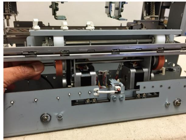
7. Place the new Shaft into the Drive Panel Steering Sub Assembly.
