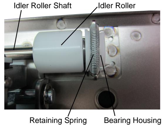
4. Remove the Idler Roller with the Bearing Housings (2) from the Bushing Forks.
