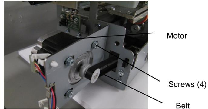
5. To replace the Alignment Stepper Mount Bracket
