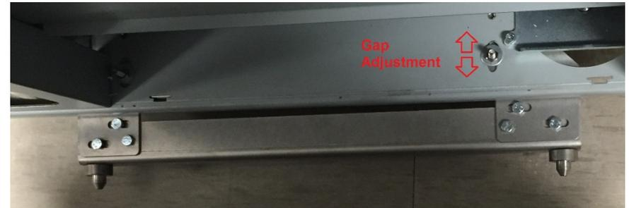
6. After the Gap adjustment has been made, dock the eWire to the upstream device again and confirm the spacing is correct. You may want to mark the position on the eWire frame so you can return to it later if needed.
