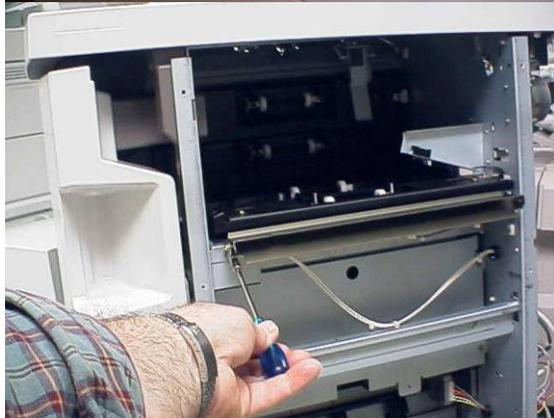
Before the system can be docked correctly the paper guide on the finisher needs to be removed. This is not used on the finisher when in line with the StreamPunch.
