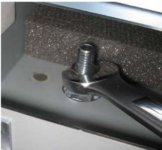
Using a 9/16" (15mm) open ended wrench, loosen the jam nut(s) situated on the caster stud inside of the machine.
