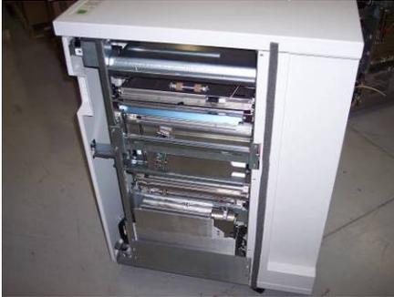
Apply one of the two remaining long strips to the right side of the printer side of the StreamPunch as shown.
