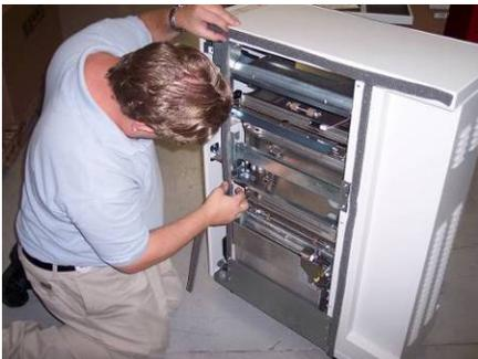
Apply the last remaining long strip to the left side of the printer side of the StreamPunch as shown.
