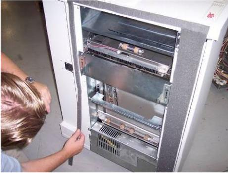
Apply one of the three longer strips to the left rear panel as shown.
