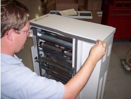
Apply the last remaining short strip to the top cover edge of the printer side of the StreamPunch as shown.
