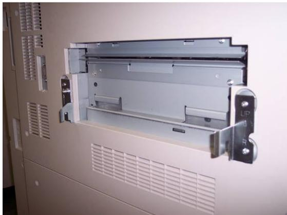
Install as shown with the bracket marked "R" on the right side facing you as you look at the exit side of the upstream device. Install the bracket marked "L" on the left side facing you. Both brackets should be oriented with the arrow facing up.
