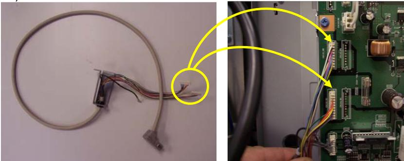
Replace the finisher to printer cable with the longer cable provided. Plug the 8 & 9 pin connector's into CN100 & CN101 on the finisher board. Replace the finisher rear cover.
