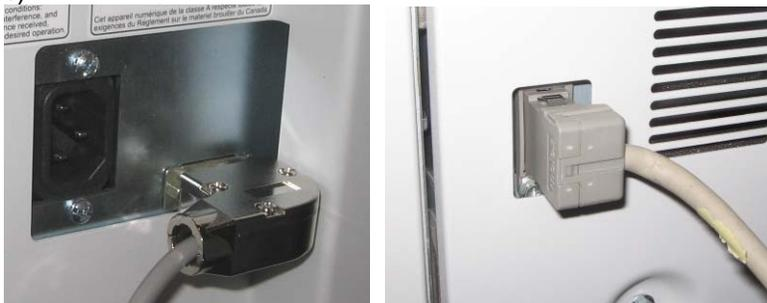
Plug the free end of the cable from step a) into the right side of the StreamPunch. Plug the free end of the cable from step b) into the connector on the printer.
