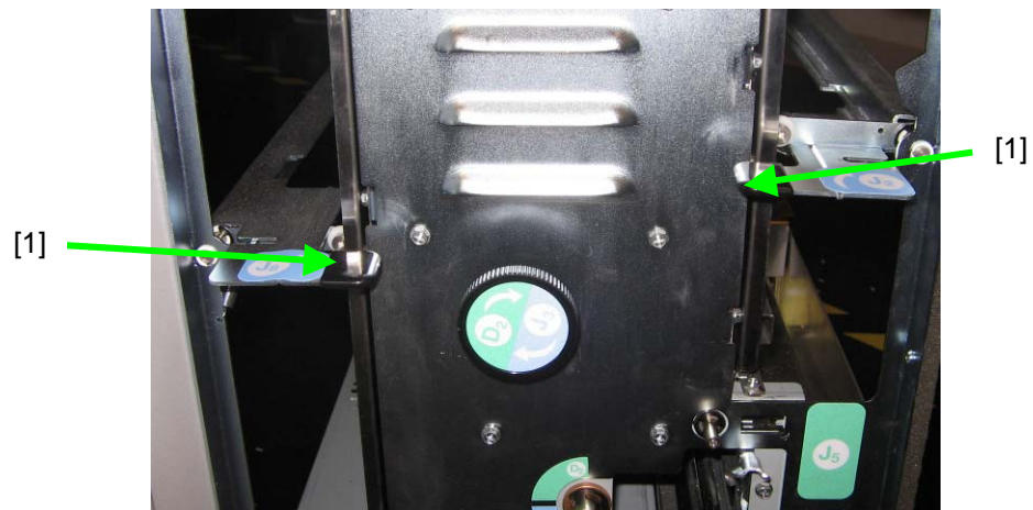
Figure 1.26 Open and Close Aligner Panel Latches.
