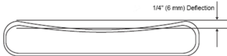
Figure 4.76 Typical Belt Deflection.
