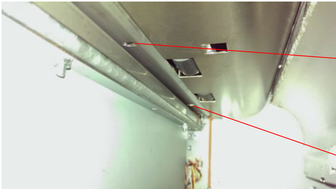
Sensors S16 and S17 are on Backgage Sensor Board.
