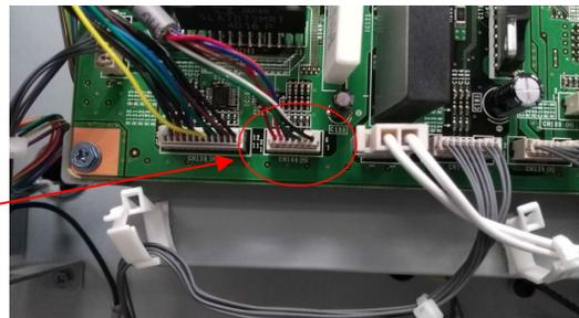
CN144 is located near the bottom left of the control board.
