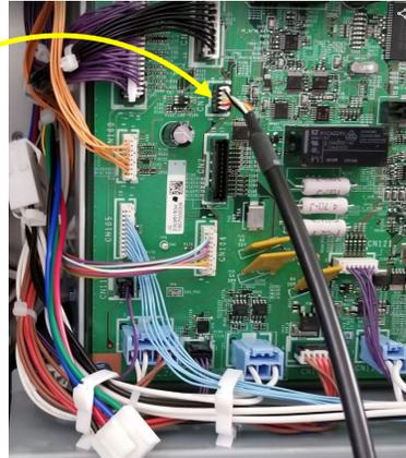
CN109 is located on the left side of the Finisher's control board
