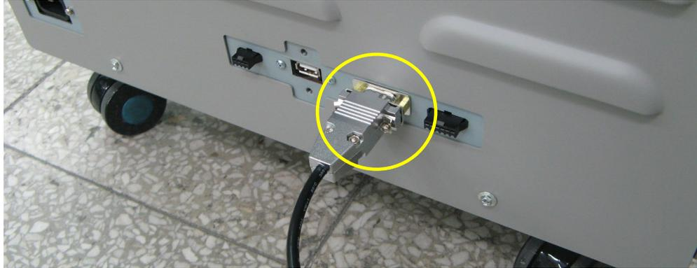
c) Replace the finisher rear cover and make sure the finisher cable is plugged in. Ensure that the communication cables are not pinched anywhere.
