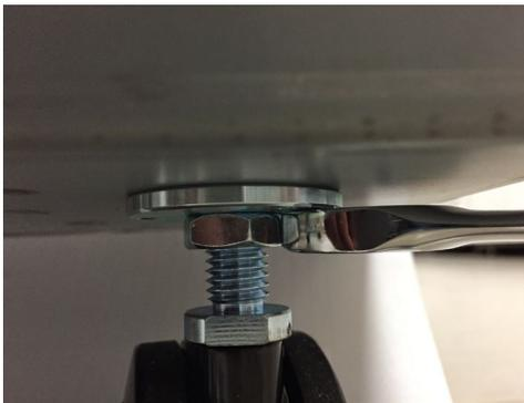
Using a 19mm (3/4") open ended wrench, loosen the jam nut(s) situated on the caster stud under the base of the machine.
