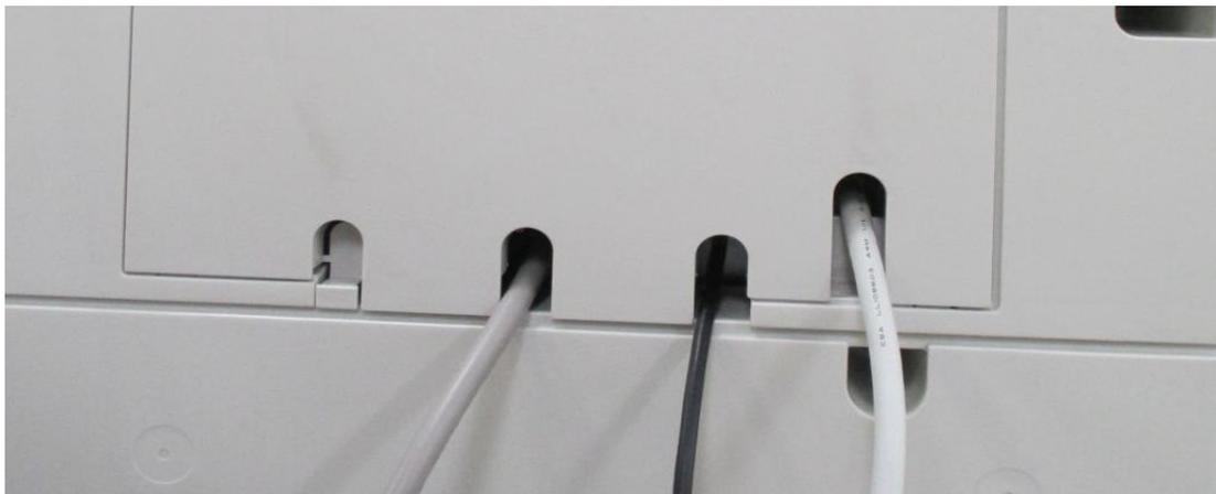
d) Connect the supplied AC power cable to the SmartPunch Plus on the rear side lower left corner. SmartPunch Plus has a power switch on the front of the machine. Ensure this is turned on.
