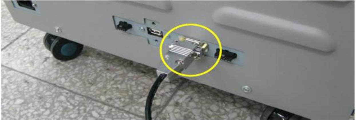
c) Replace the finisher rear maintenance cover. Ensure that the communication cables are not pinched anywhere.
