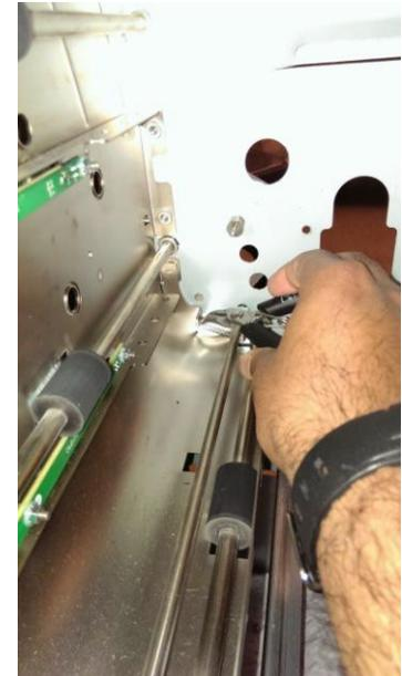
5. Remove the M3 screws (2) from the Accel Idler Panel Front and Rear Latches.
