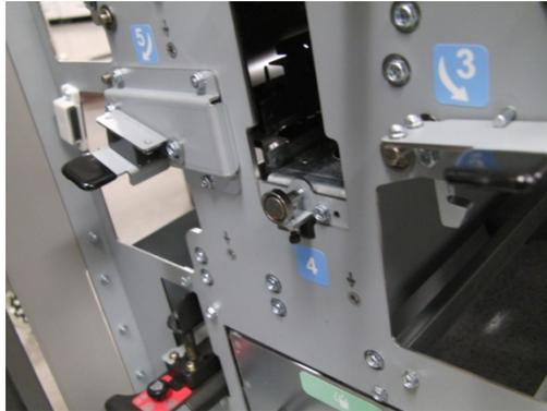
3. Loosen the Nut and Lock Screw.
