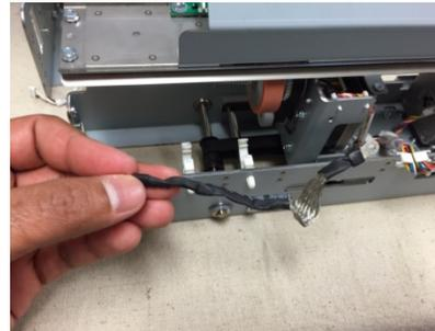
8. Remove the Steering Carriage Ground Strap.
