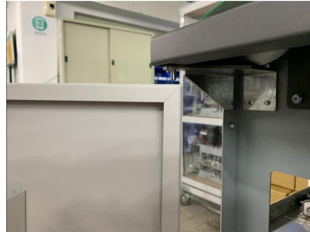
2. Insert the bottom door pin into the Front Door Bottom Hinge Bracket
