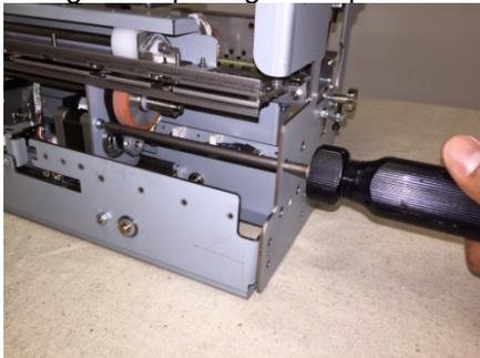
However to remove the rear side steering motor, Alignment stepper motor sub-assembly needs to be removed- ARP 3.8
