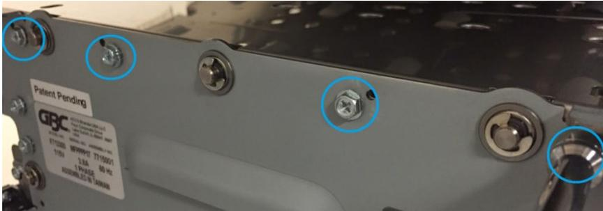
4. Remove (4) M4 screws from the Rear frame.
