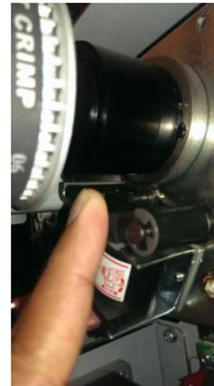
5. Check the tightness of (2) cone point set screws in the clutch.
