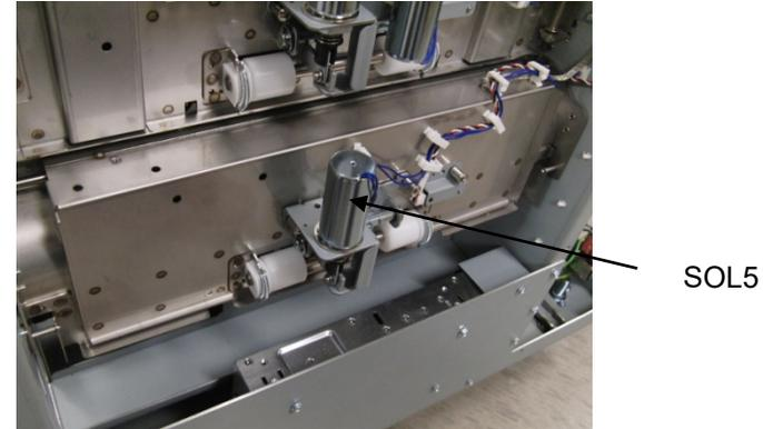
5. Open the Cable Clamps and remove the Cable.
