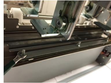
6. Place the new Backage Sensor Board in position.
