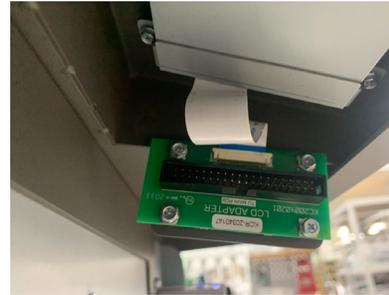
**Cable 7724421 is connected at the adapter PCB.**
