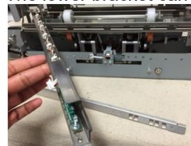
10. To replace the upper bracket, remove the cable clamps, cable, Alignment sensors, washers, nuts from the old bracket and transfer them to the new bracket.
