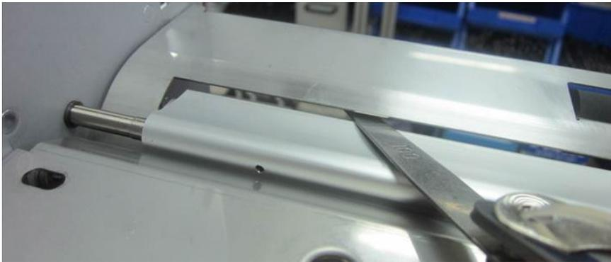
The clearance should be minimum 1.0 mm.
