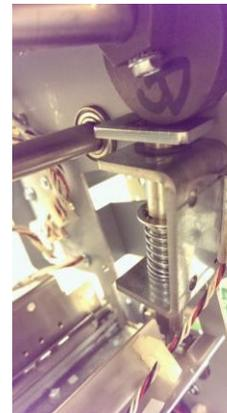
7. Inspect the surface of the cam and cam follower pad, if there is any debris, clear it.
