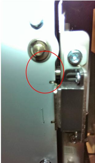
3. When the idler panel is opened and closed, you should be able to see the Idler springs extend, which will ensure proper idler roller pressure.
