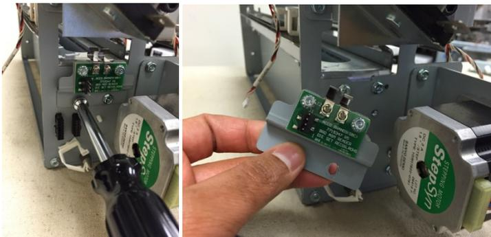
7. Remove the (2) Screws from the front and (2) screws from the back that hold that Die Rail Assembly.
