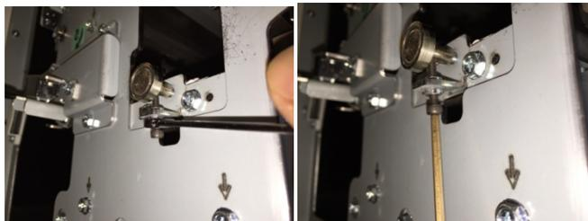
4. Rotate the Die Set Magnet to adjust the position of the Die Set Stop.
