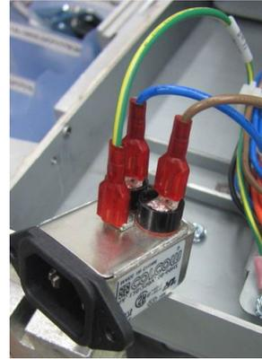
5. Remove the Wires (3) and the AC Filter.
