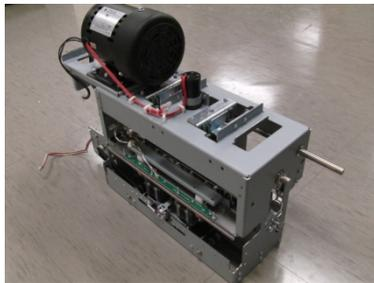
6. Remove the Shoulder Screw from the hole in the Shaft at the rear of the Punch Module.
