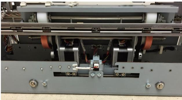
5. Remove the E-Rings (2), the Spring, the Steering Drive Roller and the Flat Washers (2) from each end of the Shaft.
