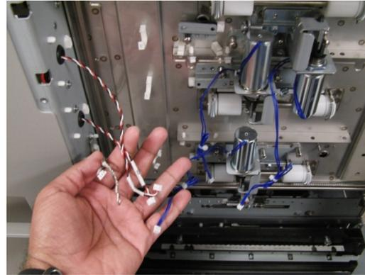
7. Disconnect the Connectors for Solenoids SOL6, SOL7, & SOL8 from the header at the rear frame.
