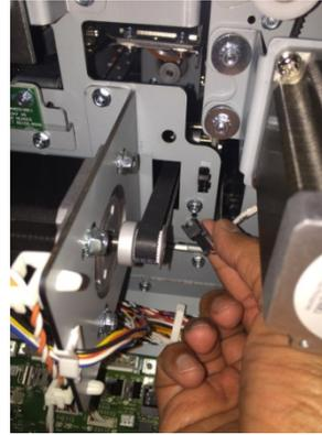
11. Disconnect the Connector for Solenoid SOL2.
