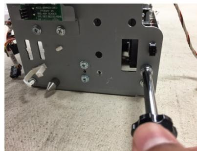
11. Remove the Steering Module from the Punch Module, by tilting the Steering Module as shown. This is to ensure the back side clears the self-clinching nut.
