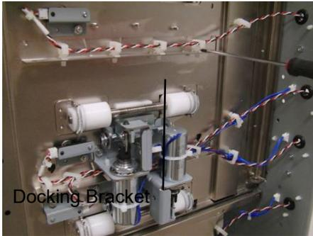
5. Disconnect the Connectors for Sensors S2, S3, & S4.
