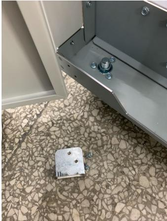
4. Lower the Door down off the pin on the Front Door Top Hinge Bracket.
