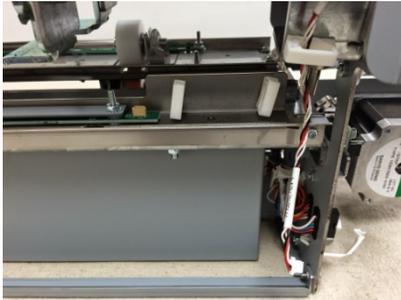
6. Remove the Screws (2) that hold the Dieset Recognition Bracket.
