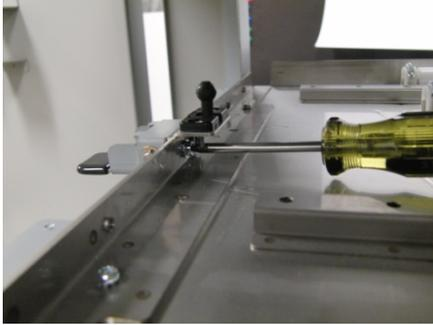
9. Remove the Idler Panel Mount Bracket from the rear frame.
