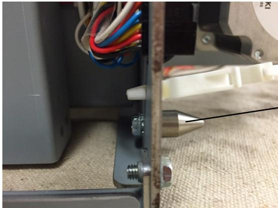
5. Place the new Mount Pin in position and tighten the Screw.
