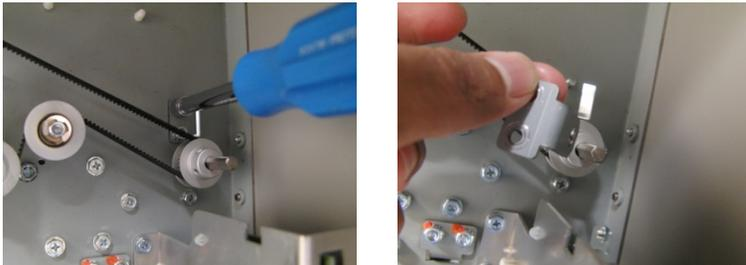
10. Remove the Upper Bypass Assembly.
