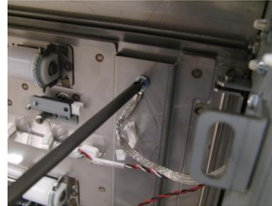
7. Disconnect the Connectors for Solenoids SOL3 & SOL4 from the header.
