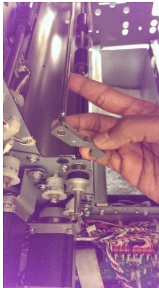
10. For the Accel Idler Panel Front Latch Assembly, slide the shaft towards the rear side to remove.
