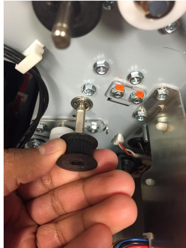
6. Place the Timing Pulley in position on the Shaft and install the retaining ring.
