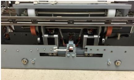
Note: There is no need to remove the Steering module if you have a screwdriver or a 5.5mm nut driver that will reach the (4) screws through the opening in the punch frame.
