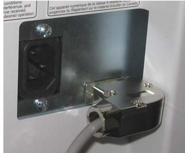
b) Plug the appropriate power cord into the side of the machine next to the communication connector. The exact location can be seen in the above picture. Insert the plug into the power supply socket.
