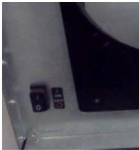
The power switch for the SmartPunch Pro can be found on the front frame on the lower left corner (shown left). Turn the SmartPunch Pro on before the main unit.
