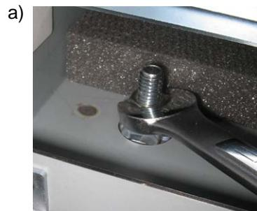
Using a 9/16" (15mm) open ended wrench, loosen the jam nut(s) situated on the caster stud inside of the machine.
