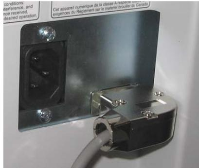
b) Plug the appropriate power cord into the side of the machine next to the communication connector. The exact location can be seen in the above picture. Insert the plug into the power supply socket.
