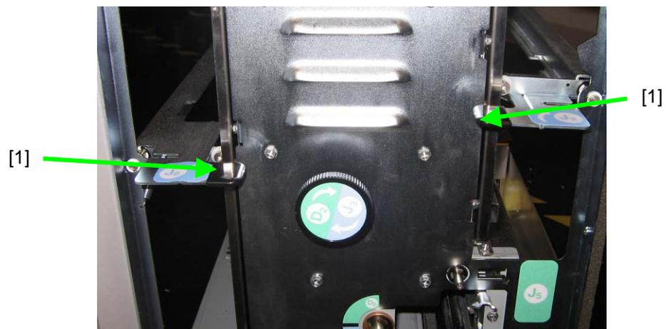
Figure 1.26 Open and Close Aligner Panel Latches.
