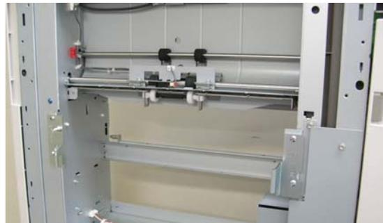
The docking bracket(s) provided with the finisher should be attached to the downstream side of the SmartPunch Pro with (4) M4x10 size screws.
