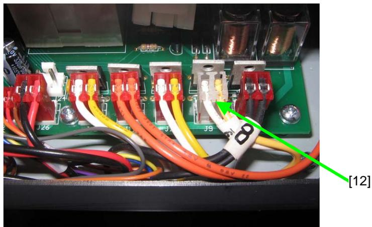
Figure 4.62 Punch Clutch Connector on the Control Board.
