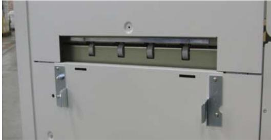
Install as shown with the bracket marked "R" on the right side facing you as you look at the exit side of the upstream device (pictures shown). Install the bracket marked "L" on the left side facing you. Both brackets should be oriented with the arrow facing up.
