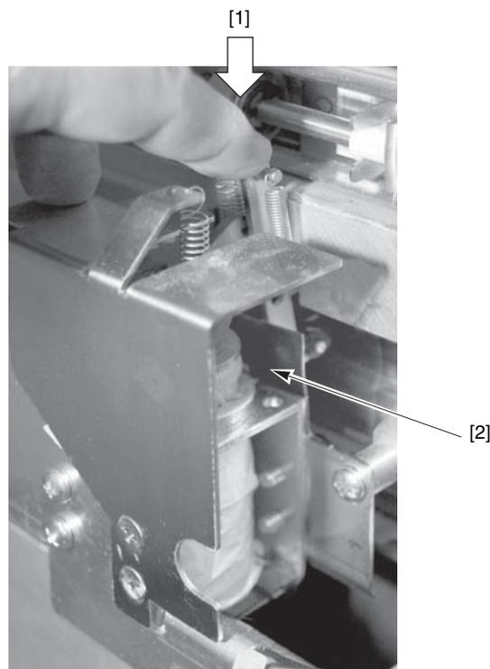
Figure 1.15 Inspect and Clean Back Gauge Solenoid.
