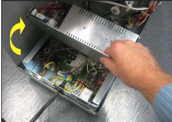
Figure 4.36 Exposure to Circuit Board
