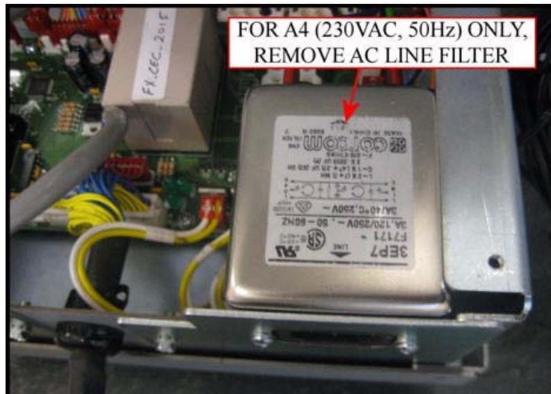
Figure 4.38 Removal of AC Line Filter
