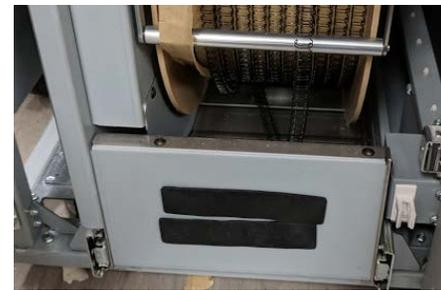
Example of improper magnet storage:
