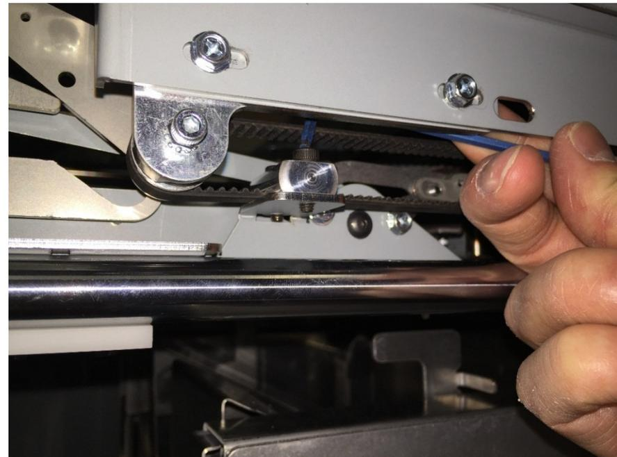
6. Slide the Timing Belt off the Pulleys and remove the Timing Belt.
