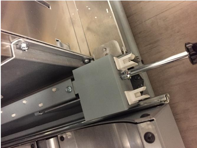
5. Remove the wires from the appropriate Interlock Switch. Note the orientation of the wires before disconnecting.
