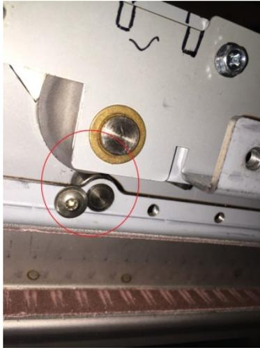
8. Ensure the encoder disc is properly positioned in relation to S48 Closer encoder sensor
