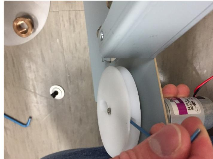
18. Remove the Spool Rewind Motor M8 by removing the #4-40 Screws securing it to the Element Feeder.
