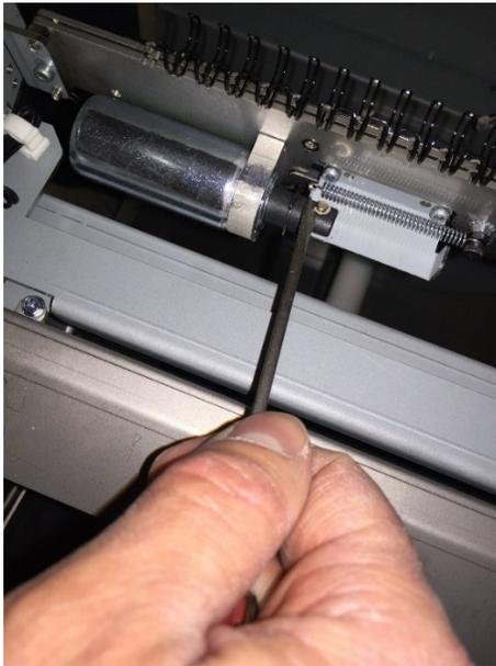
1. Insert the new Solenoid into the Solenoid Clamp and position it to the Holder Lock Assembly. Secure the Solenoid Clamp using the M3 Screw.
