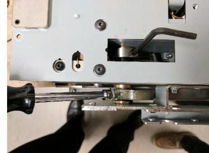
6. Before tightening the collar, using a hex key, apply counter-clockwise torque to the collar. This ensures that there is no slack on the top section of the chain. While holding the chain taught, secure the M4 set screw. One must apply significant torque to properly tighten the collar. A nut-driver (pictured below) can help.
