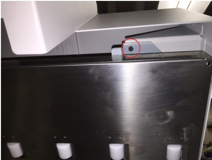
5. Remove the Socket Head Screws (2) that secure the back half of the Top Cover. There is a screw on each arm.
