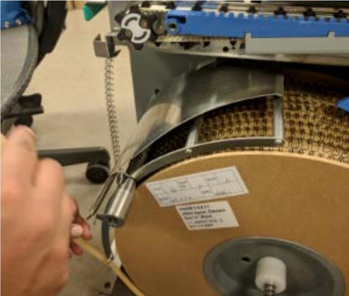
10. Lift the metal guide of the shield and slide the carrier paper between it and the lower bars.
