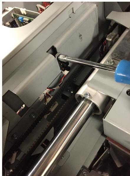
8. Remove the Closer Home Sensor S46 by removing the M3 Screw.
