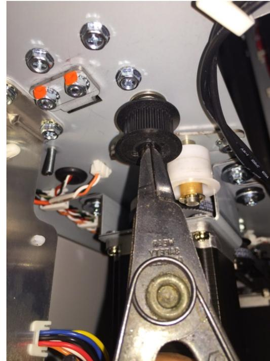
6. Remove the Timing Pulley by sliding it off the shaft.
