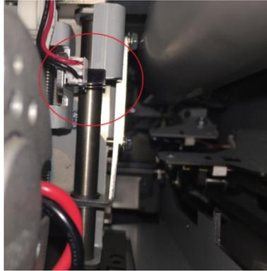
8. Inspect the closer jaw springs and ensure they are positioned correctly.
