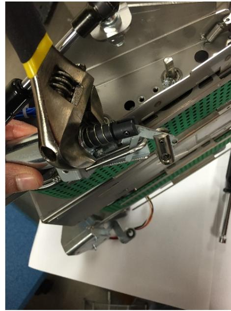
11. Remove the Kick-Down Solenoid Assembly from the Vacuum Stacker.
