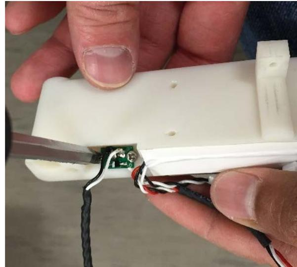
10. Remove the M2 Screws (2) to remove the Emitter PCB.
