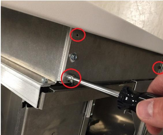
5. Remove the M4 Screws (3) from the right side cover plate, while holding the cover plate secure with your free hand. Remove the cover plate and set it aside.
