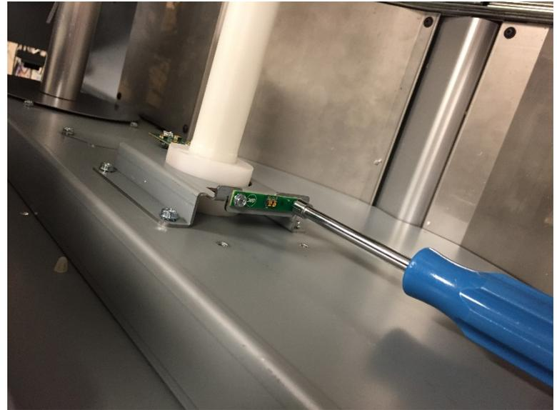
7. Disconnect the Sensor Cable from the back side of the PCB.
