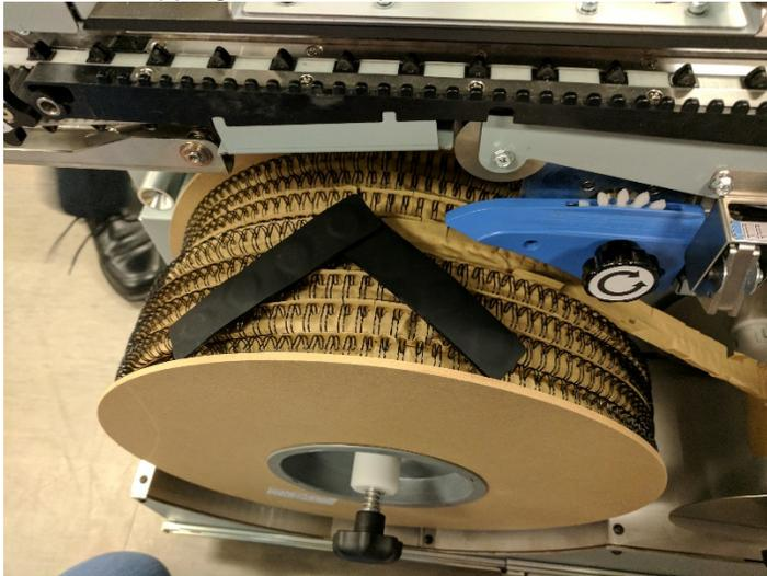
9. Tear the carrier paper where it leaves the rewind spool. Your carrier paper should extend about 12 inches (30 cm) beyond the loose end of your wire.
