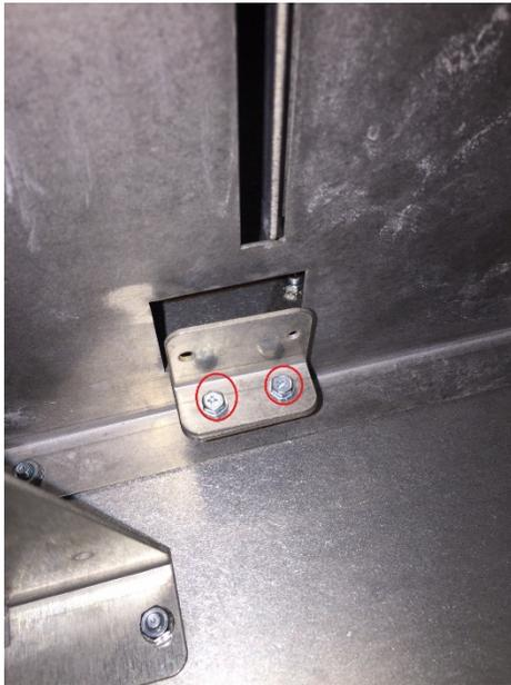
7. Disconnect the Sensor from the bracket by removing the M3 Screw and remove the old sensor.
