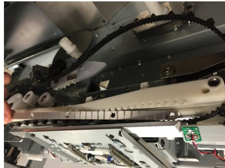
11. Remove the Element Feeder Belt.
