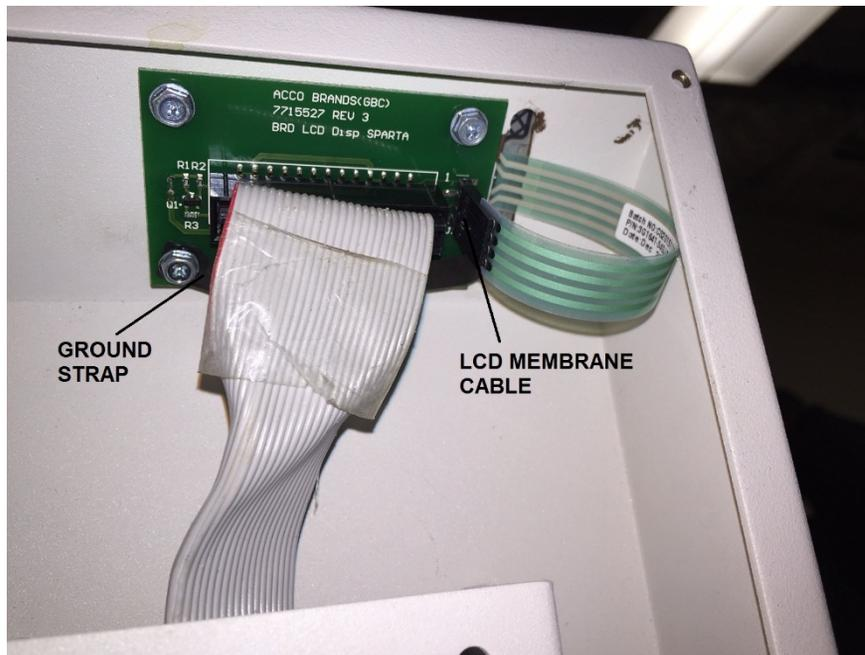
5. Remove the M3 Screw that secures the ground strap.
