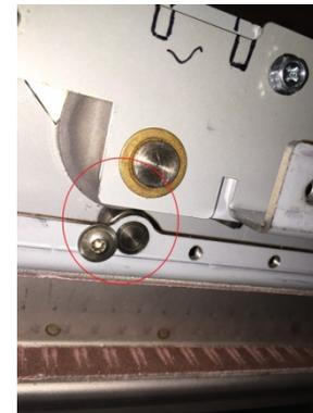
7. Ensure the sheet metal feature properly blocks/unblocks S47 Closer full open sensor
