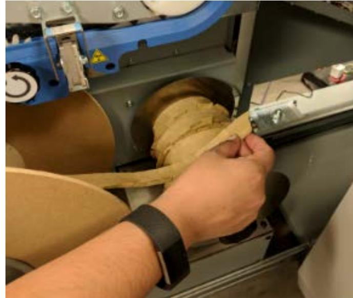
10. Unscrew the spool retainer. Turn the knob counterclockwise to loosen and remove the cap. Set the cap aside.
