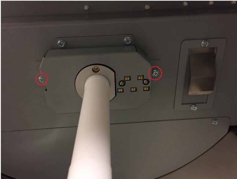
6. Remove the M3 Screws (2) and remove the Spool Empty PCB from its mounting bracket.
