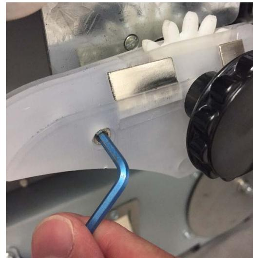
8. Remove the Sprocket Nose Sub-Assembly from the Element Feeder.
