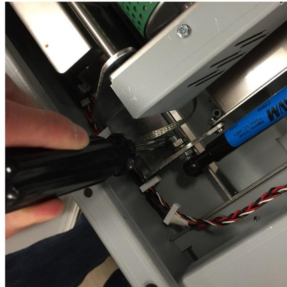
22. Repeat the procedure to remove the M4 Screws (2) from the rear hinge bracket.
