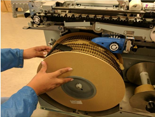
12. To remove the rewind spool from the feed spindle, push the hub in and turn it clockwise. Remove the excess paper by sliding it off the hub. If the rewind spool is full of paper, it may be difficult to remove. The spool must be pressed in firmly before rotating to disengage the pin. Reinstall the empty Paper Feed Hub onto the spindle.
