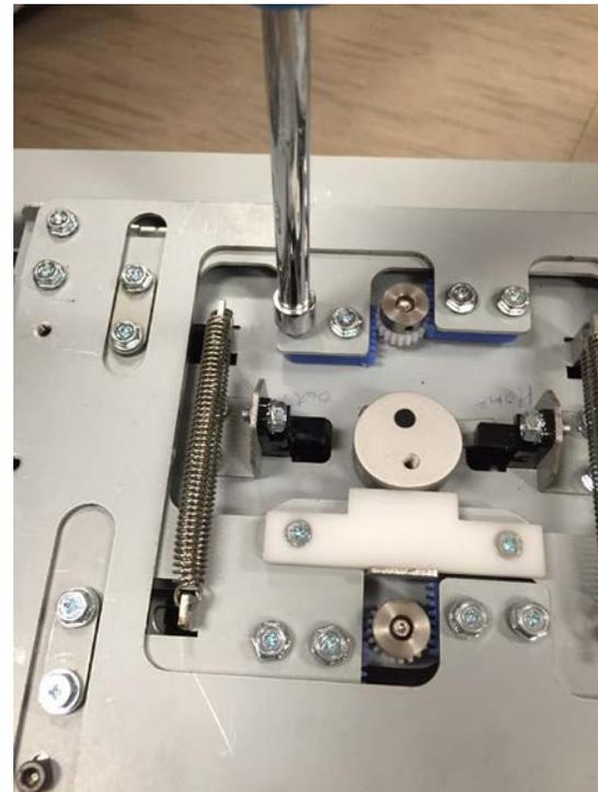
5. Carefully remove the Rack by sliding it out of the module.
