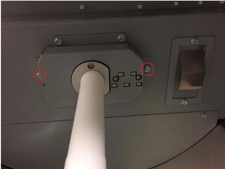
6. Remove the M3 Screws (2) and remove the Spool Detect Sensor PCB from its mounting bracket.
