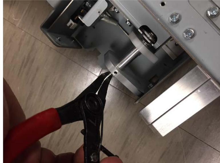
6. Loosen the set screw securing the Cam to the Shaft.
