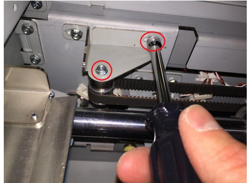
5. Remove the M4 Screws securing the Timing Belt Clamp, and remove the Timing Belt Clamp.
