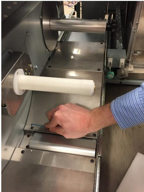
10. Remove the M4 Screws (8) securing the Spindle Frame Assembly to the Element Feeder. Carefully tilt the Spindle Frame Assembly forward to remove it from the Element Feeder Body.
