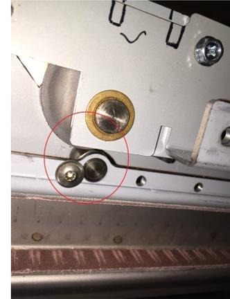
9. Ensure the encoder disc is properly positioned in relation to S48 Closer encoder sensor
