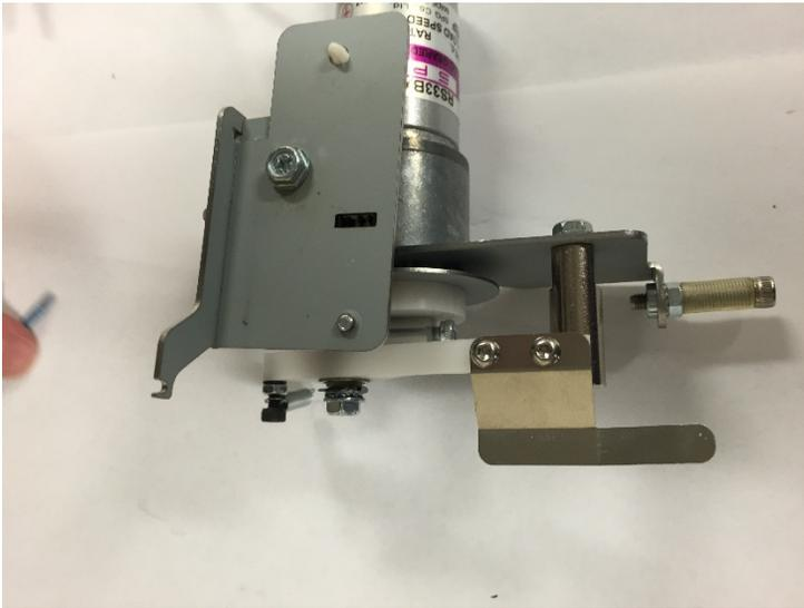
3. Ensure that the Disk Encoder is approximately centered in the Tapper Front Sensor. If it is not centered, loosen the set screw and adjust the Hub until it reaches the correct position and re-tighten the set screw.
