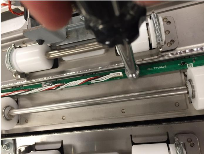
10. Remove the old Skew Sensor PCB from the Upper Bypass.
