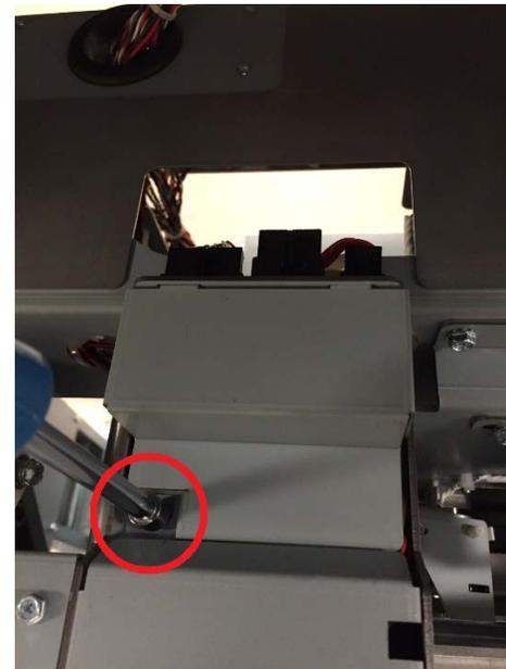
7. Remove the M4 Screws (2) from the back of the Deflector
