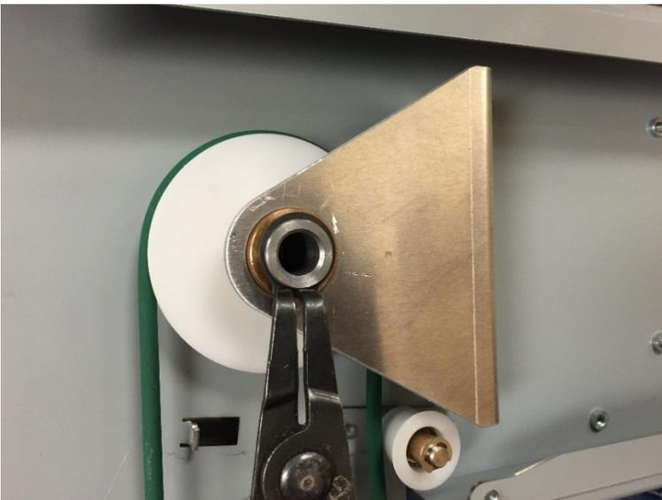
13. Loosen the M4 Set Screw securing the Idler Pulley to the Rewind Spool Shaft, and slide the Idler Pulley off of the Shaft.
