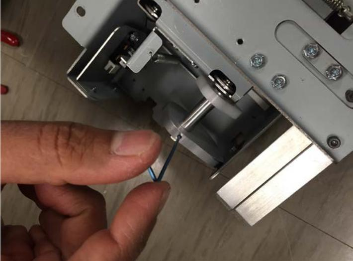
7. Slide the Cam and Washers off the shaft.
