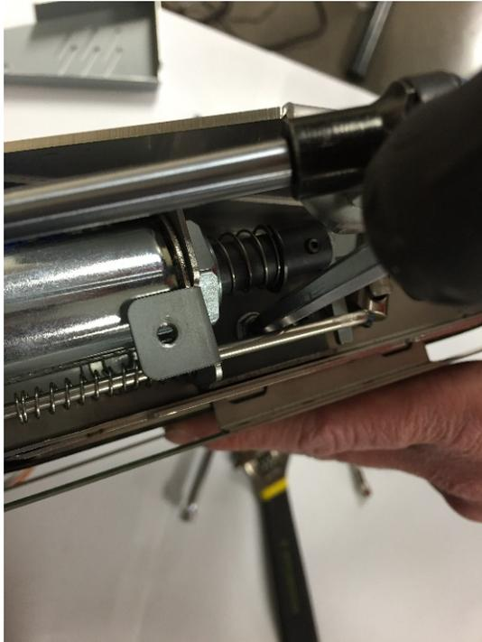
10. Use an adjustable wrench to loosen the nut securing the Solenoid to the bracket.
