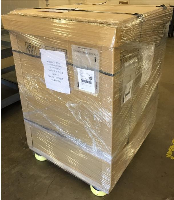
3. Remove the plastic shrinkwrap from the container and remove the Packing Straps.
