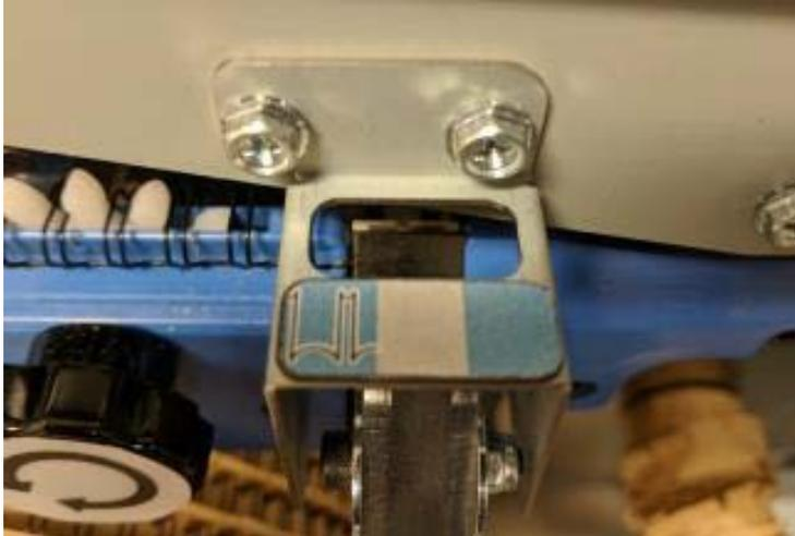
14. Confirm that the spool is installed properly.
