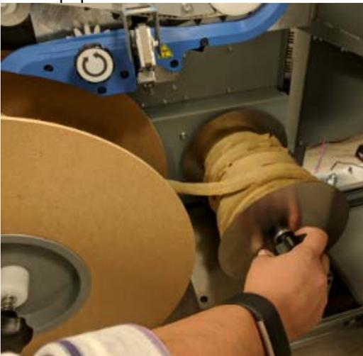
4. Lift the metal wire guide on the shield and pull the carrier paper out from the shield. Then Remove the wire shield. Pull on the wire shield handle to remove the entire shield, and place the shield safely on top of the element feeder.
