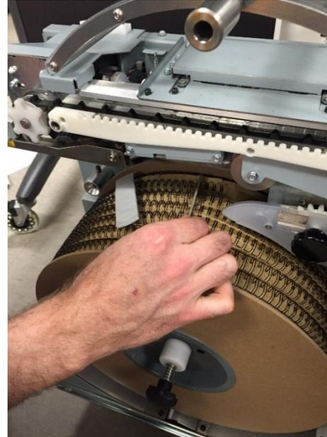
8. Pull the wire and paper away from the spool and hold them both in one hand. With your free hand install the wire shield.
