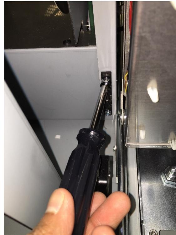
4. Locate the female half of the Latch on the bracket near the back of the Frame. Remove the Latch by removing the M3 Screws (4).
