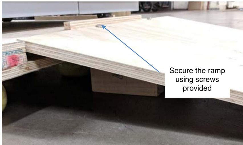
14. Using two people, carefully push the eWire from the back down the ramp. Make sure the eWire casters stay on the pallet and the ramp and control the machine on the way down. Make sure to support the eWire carefully while moving due to its weight.
