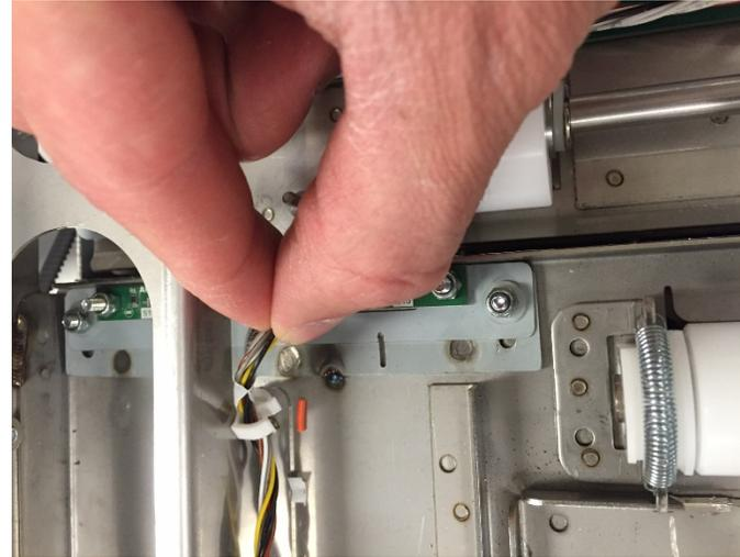
6. Release the Alignment Sensor PCB by removing the M3 Nuts (2)
