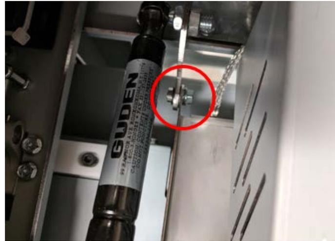
21. Remove the M4 screws (2) from the front hinge bracket.
