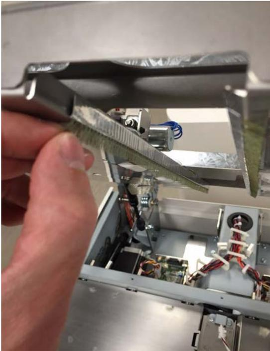
5. Use a cloth and alcohol to remove any adhesive residue from the surface.
