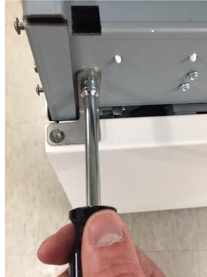
5. Lift the Door up off the pin on the lower hinge bracket.
