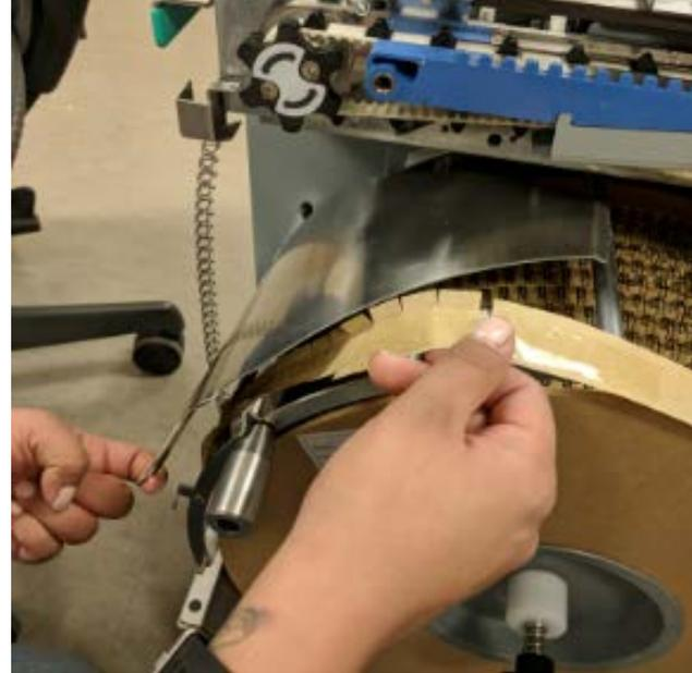
11. Attach the loose end of the support paper to the paper feed hub. Secure the paper to the hub via the metal clip.
