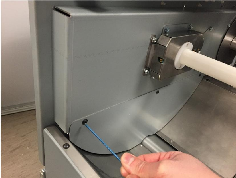
9. Remove the curved Rear Baffle by removing the M4 Screws (6)
