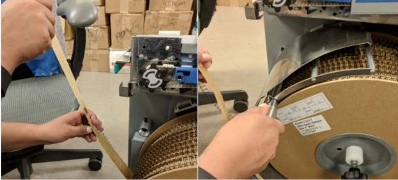
9. While still holding the carrier paper, use the magnetic catch to hold the wire.
