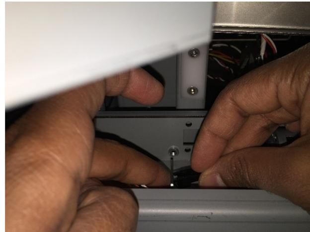
6. Remove the M4 screws (2) securing the Tapper to the eWire Frame
