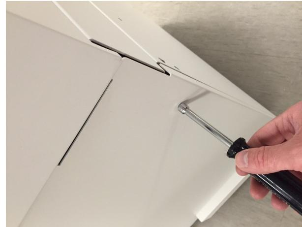
4. Carefully tilt the Back Cover back and then lift the Back Cover out of the tabs in the machine frame.
