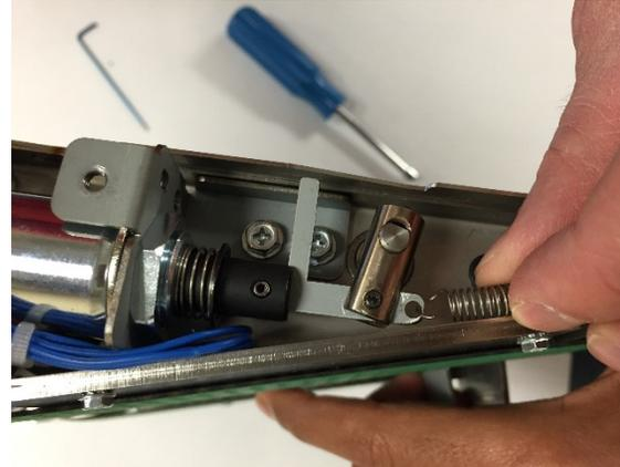
7. Loosen the set screw securing the clevis to the rotating shaft.
