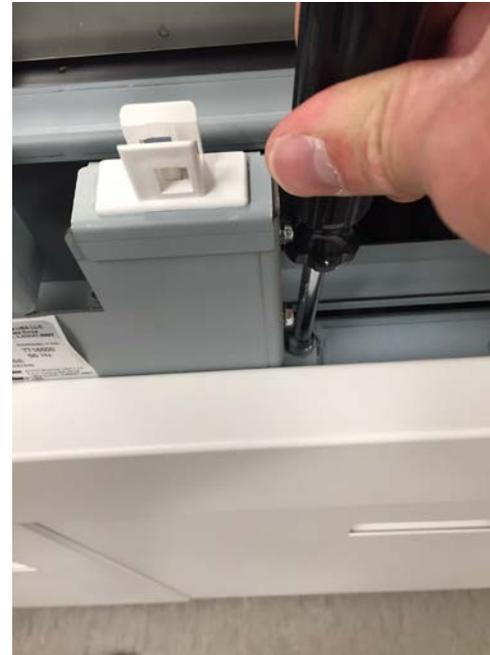
3. Close the latch by lowering the Upper Bypass Assembly fully. Ensure that the latch engages properly with the Catch. If necessary, adjust the vertical position of the Catch by loosening the Screws on the Catch Bracket and adjusting the position.
