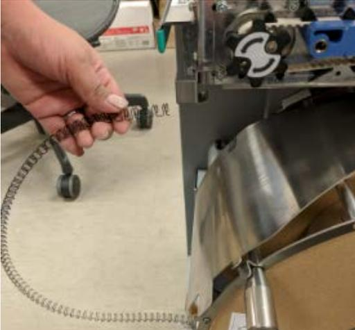
3. Turn the rewind spool counterclockwise to generate slack in the carrier paper.
