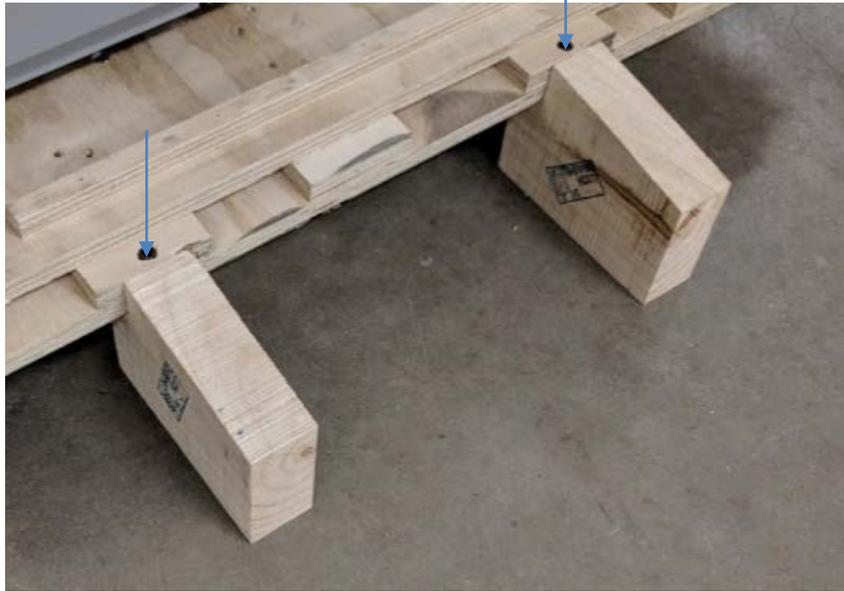
13. Place the wooden ramp onto the appropriate location on the front of the pallet. Secure the ramp in place using 2 long screws or Allen wrenches.
