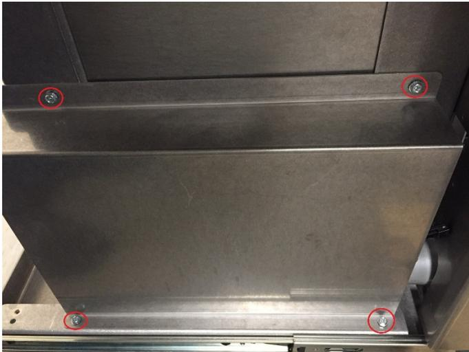
4. Remove the Sensor Bracket by removing the M4 nuts (2).
