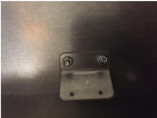
5. Remove the Sensor from the Bracket by removing the M2 Screws.
