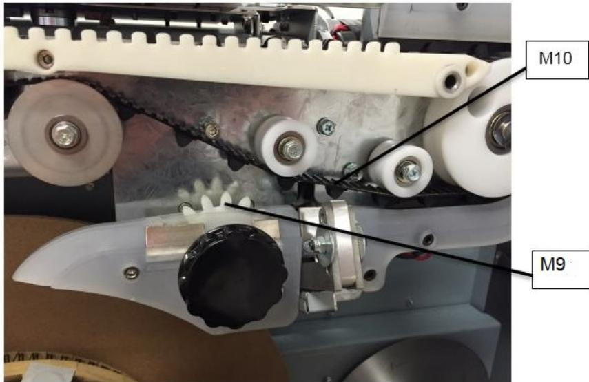
1. Do GP 6.3.5 [Motors Procedure](#) to check the motors activate as expected. M9 will rotate the Element Feed Sprocket. M10 will rotate the Element Feeder Belt.
