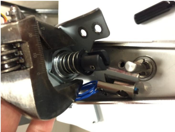
10. Remove the Kick-Down Solenoid Assembly from the Vacuum Stacker.
