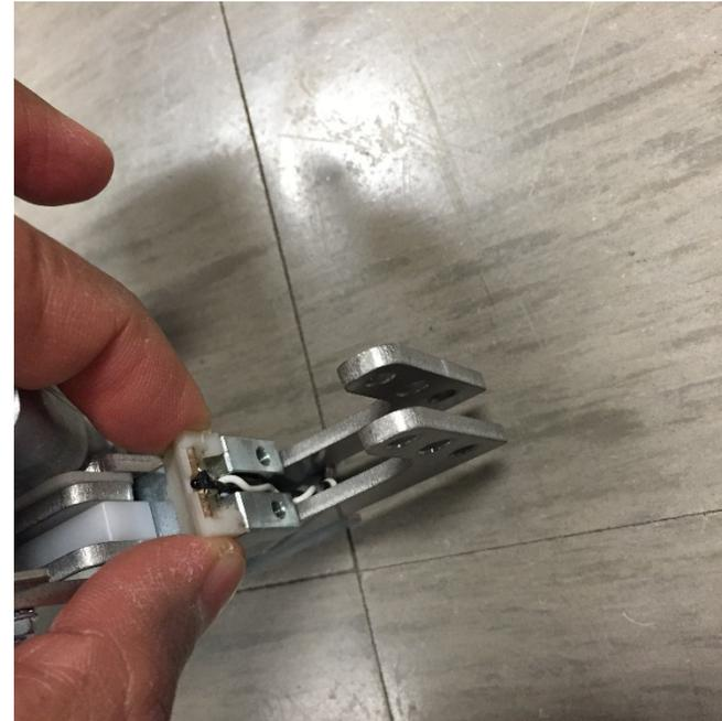
8. Remove the Upper Cable Cover by removing the M3 Screws (2).
