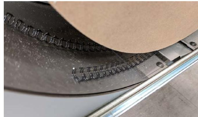
If this occurs, carefully remove the loose element/s and check the spool for damage. The most common damage occurring from this is stretched wire (see above).
