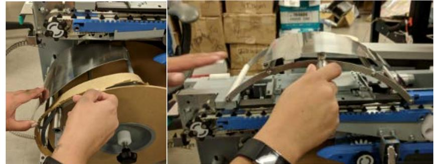
5. Rewind the spool counterclockwise to take the excess slack from the wire and the paper.
