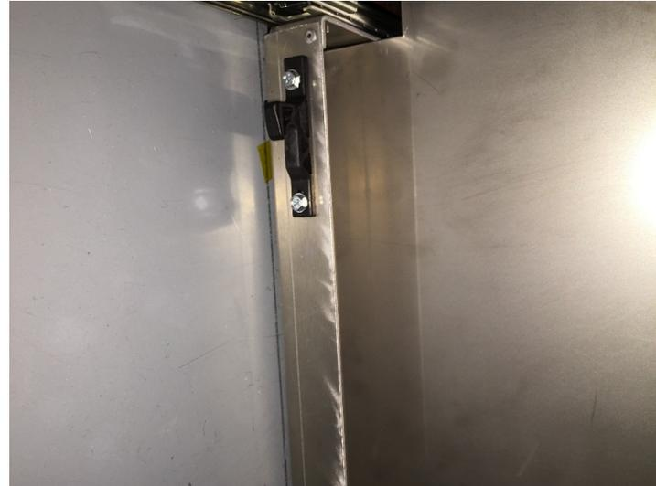
4. Locate the female half of the Latch on the bottom of the Frame. Remove the Latch by removing the M3 Screws (4).
