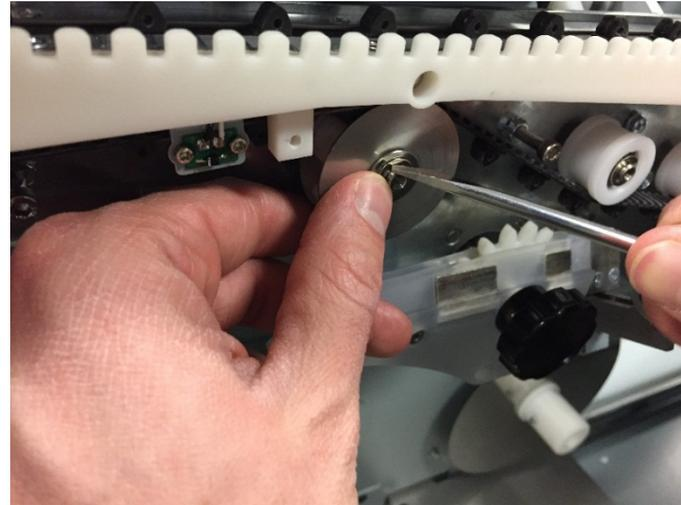
7. Slide the outermost Flange and Bearing off of the shaft and set it aside. Gently slide the plastic Idler Pulley off the shaft, carefully disengaging it from the Belt.
