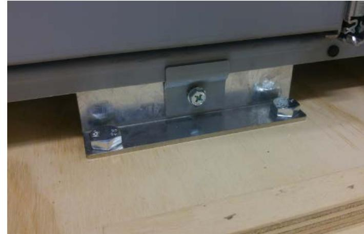
9. Repeat for the remaining Support Brackets and Bracket Clamps.
