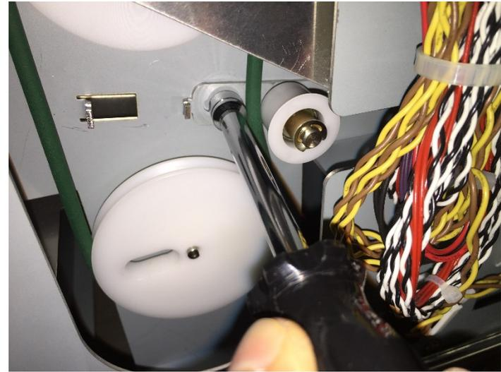
7. Slide the Belt off of the Drive Pulley.
