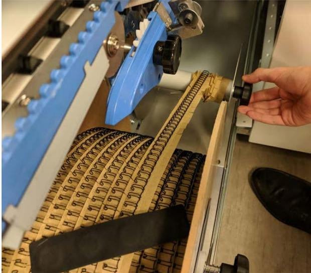
8. Secure the wire rows on the spool at the end of the loose wire using the 2<sup>nd</sup> magnet strip, then move the first magnet strip you placed as shown here. Place the magnets across rows of wire so that the loose end of wire is secured to the wound rows. The magnets prevents the wire from slipping when the spool is removed.
