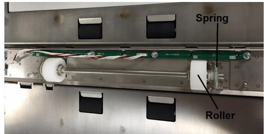
5. Slide the Idler Roller Assembly out of the Steering Module by lifting the bearings out of the bearing mount brackets
